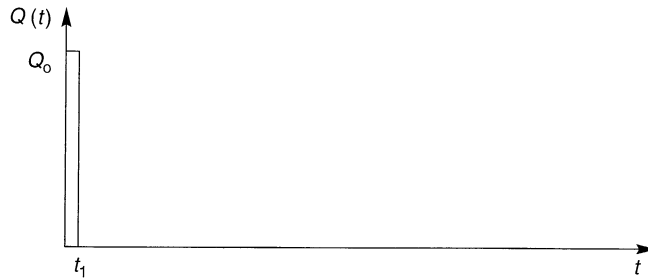
Figure B.13 Dirac pulse loading.
