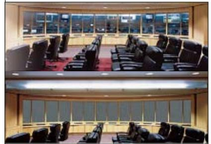
**PRIVACY GLASS** Liquid crystals have the fluidity of a liquid but the ordered structure of a solid. In privacy glass, applying an electrical charge causes the molecules to switch from a random, light-admitting arrangement to an orderly, light-blocking one.
