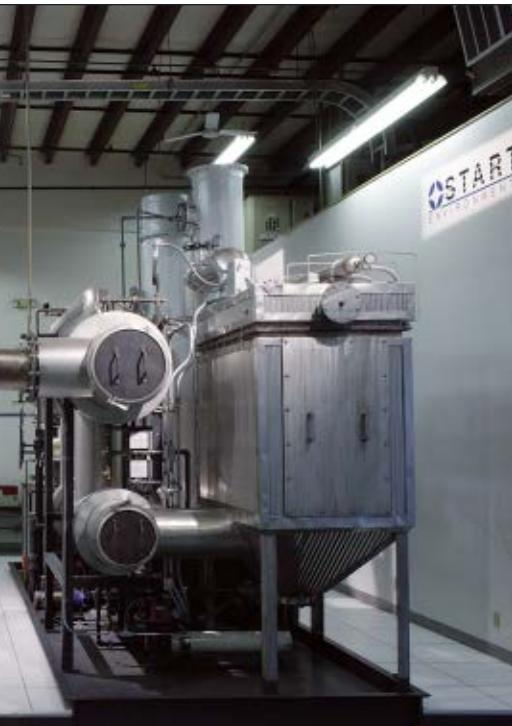
**BURN, BABY, BURN** Longo's Plasma Converter [above] is built in part from off-the-shelf components. The plasma torch contained in the vessel at left above is borrowed from the metal-fabrication world. A video screen [facing page] allows operators to see what's going on inside the burn chamber as the plasma arc rips electrons from the surrounding air. Longo [right] designed his machine to convert the syngas that results from the gasification process into hydrogen.
