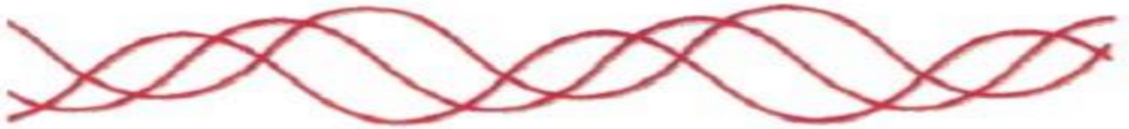
LED: one color (monochromatic) and waves not in phase (non-coherent)
