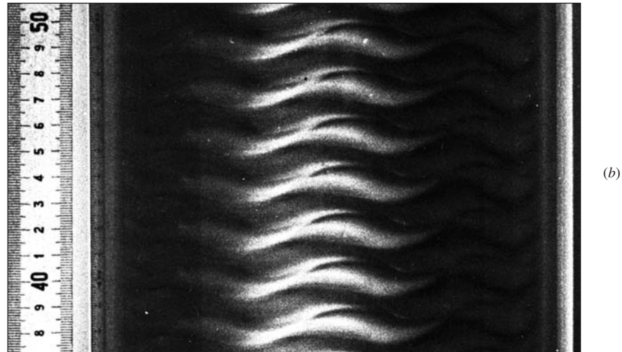
Fig. 4.14 Experimental verification of the instability of flow between a fixed outer and a rotating inner cylinder. (a) Toroidal Taylor vortices exist at 1.16 times the critical speed; (b) at 8.5 times the critical speed, the vortices are doubly periodic. (Courtesy of Cambridge University Press E. L. Koschmieder, Turbulent Taylor Vortex Flow , Journal of Fluid Mechanics , vol. 93, pt. 3, 1979, pp. 515-527. ) This instability does not occur if only the outer cylinder rotates.
