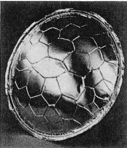
Figure 6-6. Wrinkle Pattern Identified as Turtle Backing of Solid Forward-Domed Rupture Discs Due to Alternate Reverse Flexing and Stretch Against Inadequate Support. (Courtesy of Continental Disc Corporation)
