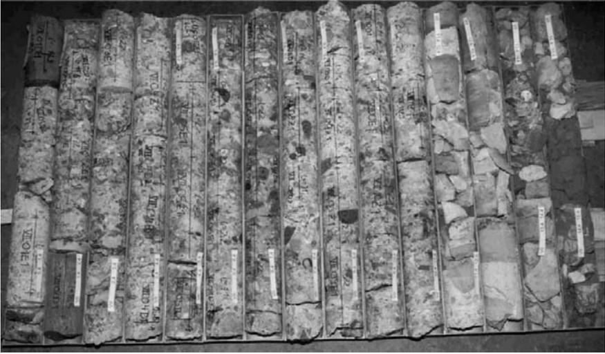
**Fig. 5-1.** Example of drilling cores. See also the marking of test specimen for material property tests
