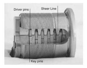
Figure 5.2 Side view cutaway.
