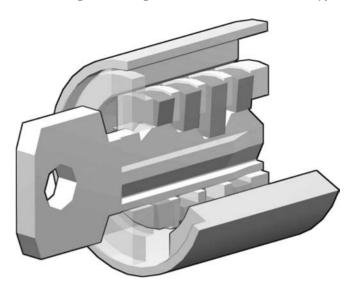
Figure 5.4 A wafer tumbler lock.
