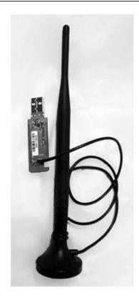
**Figure 8.7** Bluetooth adapter with hacked connecter and antenna.
