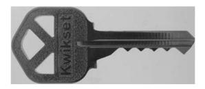
**Figure 5.18** A typical bump key.
