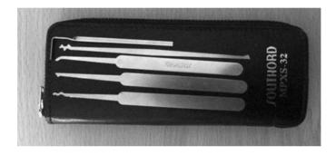
Figure 8.11 A pick set for opening pin tumbler locks.
