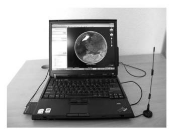
**Figure 7.3** Laptop with omni-directional antenna.
