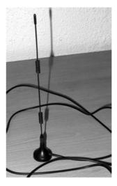
Figure 8.5 Omni antenna with 5bd gain.
