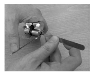
Figure 5.15 Raking a lock.
