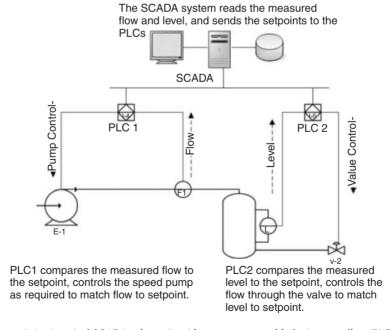
Figure 9.1 A typical SCADA schematic with two programmable logic controllers (PLCs).
