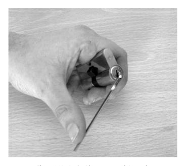
**Figure 5.12** Lock with torque wrench inserted.
