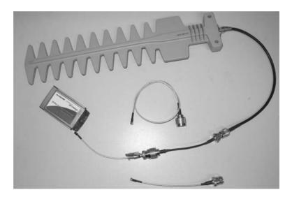
Figure 8.6 Yagi antenna with pigtail connectors.
