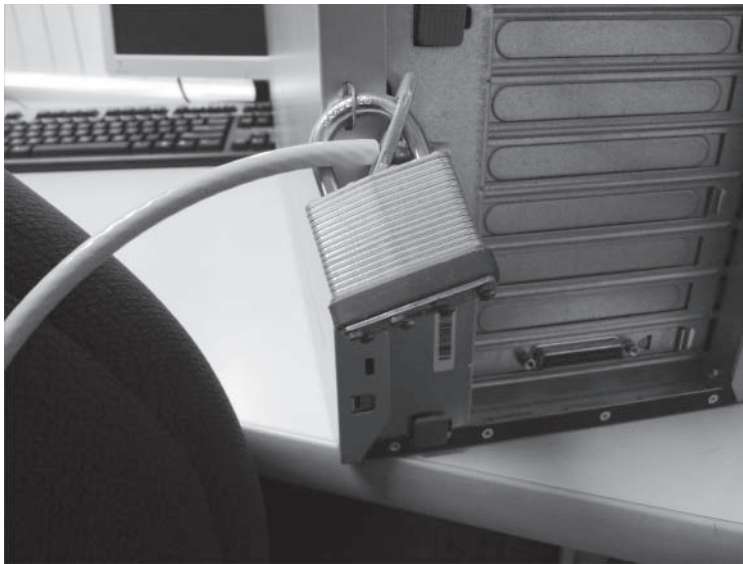
FIGURE 10.9 A cable can be used to keep a desktop machine from easily being taken.
