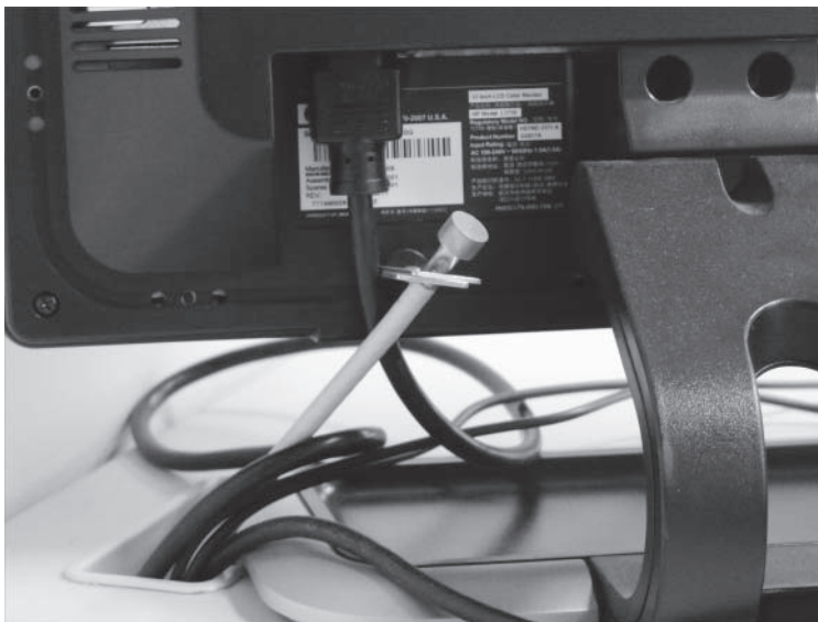
FIGURE 10.10 If theft of equipment is a possibility, run one end of the cable from the monitor to the desktop machine through the hole in the work desk.
