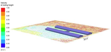
Fig. 2. Computational fluid dynamics results of natural ventilated barns separated by 30-m distance and the resulting velocity vectors at 1 m s<sup>-1</sup> in a 45° direction.
