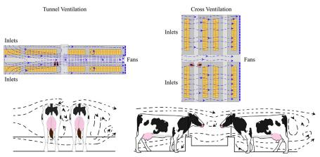
**Fig. 3.** Typical flow profiles for tunnel-ventilation (*left*) and cross-ventilation (*right*) systems; tunnel ventilation flows (*left*) parallel to the feed lane. Cross-ventilation (*right*) flows perpendicular to the feed lane.
