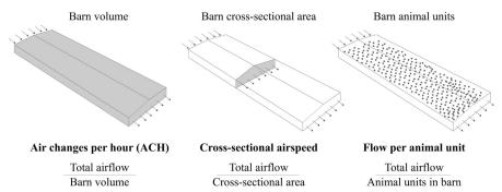
Fig. 1. Three key ventilation parameters comparing the total flow to the barn's volume, cross-sectional area, and number of animals.
