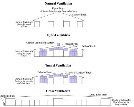
Fig. 5. Four main types of ventilation systems and their key design features.
