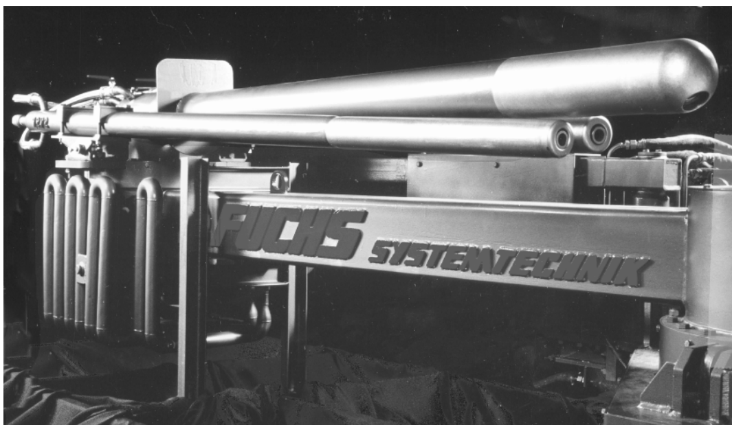
Fig. 10.18 Water-cooled oxygen lance. (Courtesy of Fuchs.)
