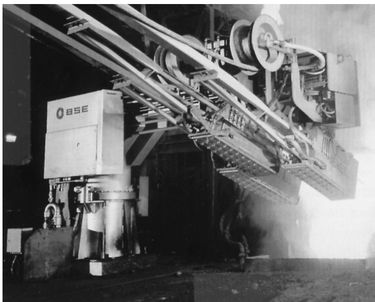
Fig. 10.17 Consumable oxygen lance manipulator. (Courtesy of Badische Stahl Technology.)
