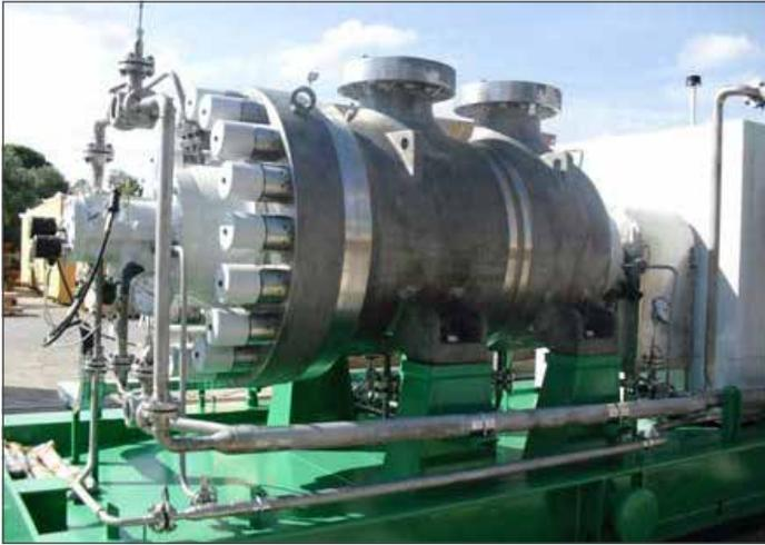
**FIGURE 16** M'Boundi main treated sea water injection pump
