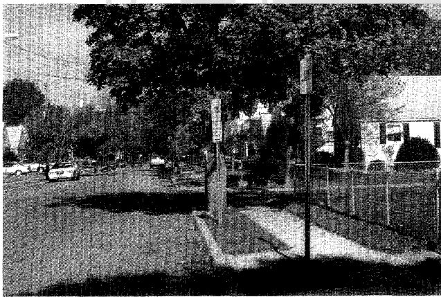
Figure 4.1: Placement of STOP Sign with Visibility Impaired by Tree
