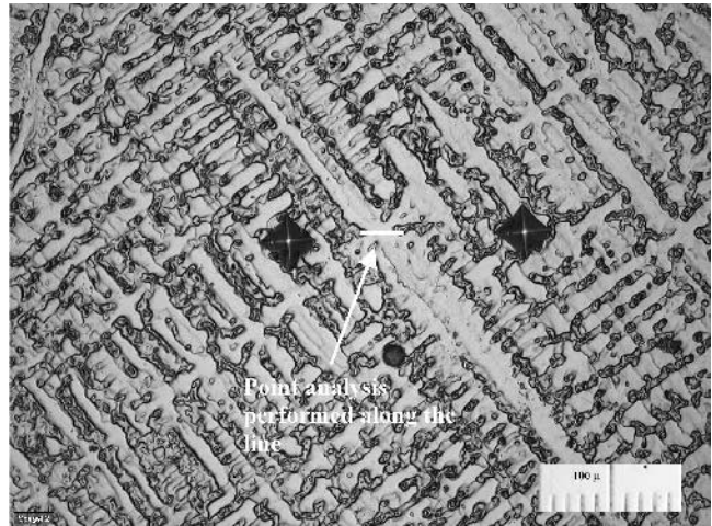
Fig. 17—The etched microstructure in a mirror furnace sample, showing a dendrite intersection and hardness marks. The chemical analysis was performed as point analysis straight across the dendrite, after removal of the etching.
