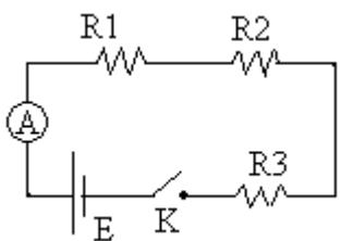
$$E=12V \text{ و } R_3=0.6\Omega \text{ و } R_1=1.4\Omega$$
