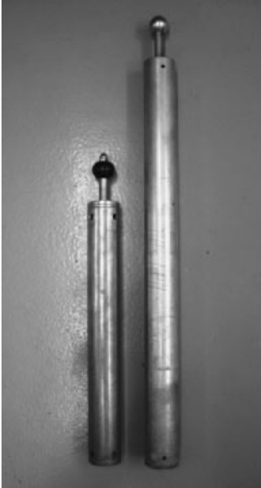
Figure 6.7 Comparison between standard Proctor hammer (left) and modified Proctor hammer (right) (Courtesy of Braja M. Das, Henderson, Nevada)
