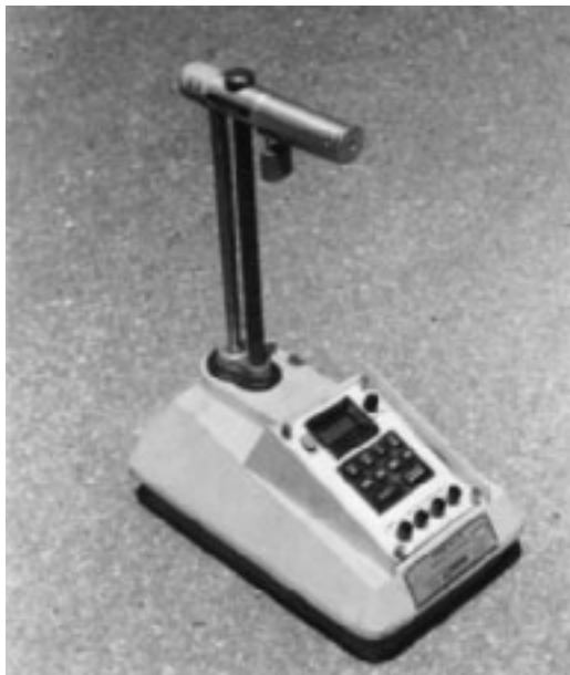
Figure 6.25 Nuclear density meter (Courtesy of Braja M. Das, Henderson, Nevada)
