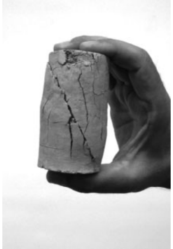
Figure 12.35 Failure by shear of an unconfined compression test specimen (Courtesy of Braja M. Das, Henderson, Nevada)
