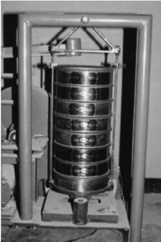
Figure 2.21 A set of sieves for a test in the laboratory (Courtesy of Braja M. Das, Henderson, Nevada)
