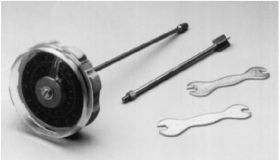
Figure 12.46 Laboratory vane shear test device ( Courtesy of ELE International )
