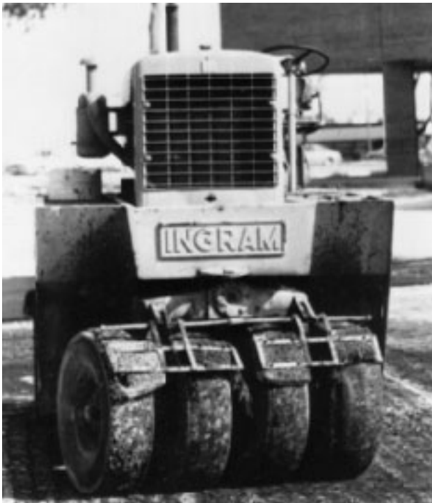
Figure 6.16 Pneumatic rubber-tired roller ( Ingram Compaction LLC )
