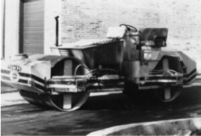
Figure 6.15 Smooth-wheel roller ( Ingram Compaction LLC )
