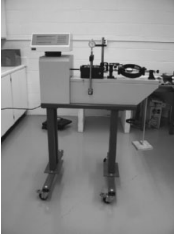
Figure 12.5 Strain-controlled direct shear equipment (Courtesy of Braja M. Das, Henderson, Nevada)
