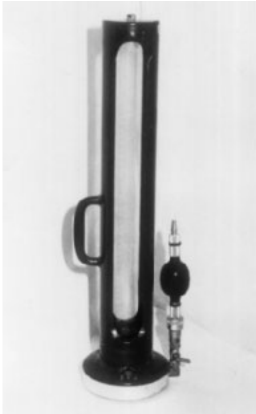
Figure 6.24 Calibrated vessel used with rubber balloon (not shown) (Courtesy of John Hester, Carterville, Illinois)
