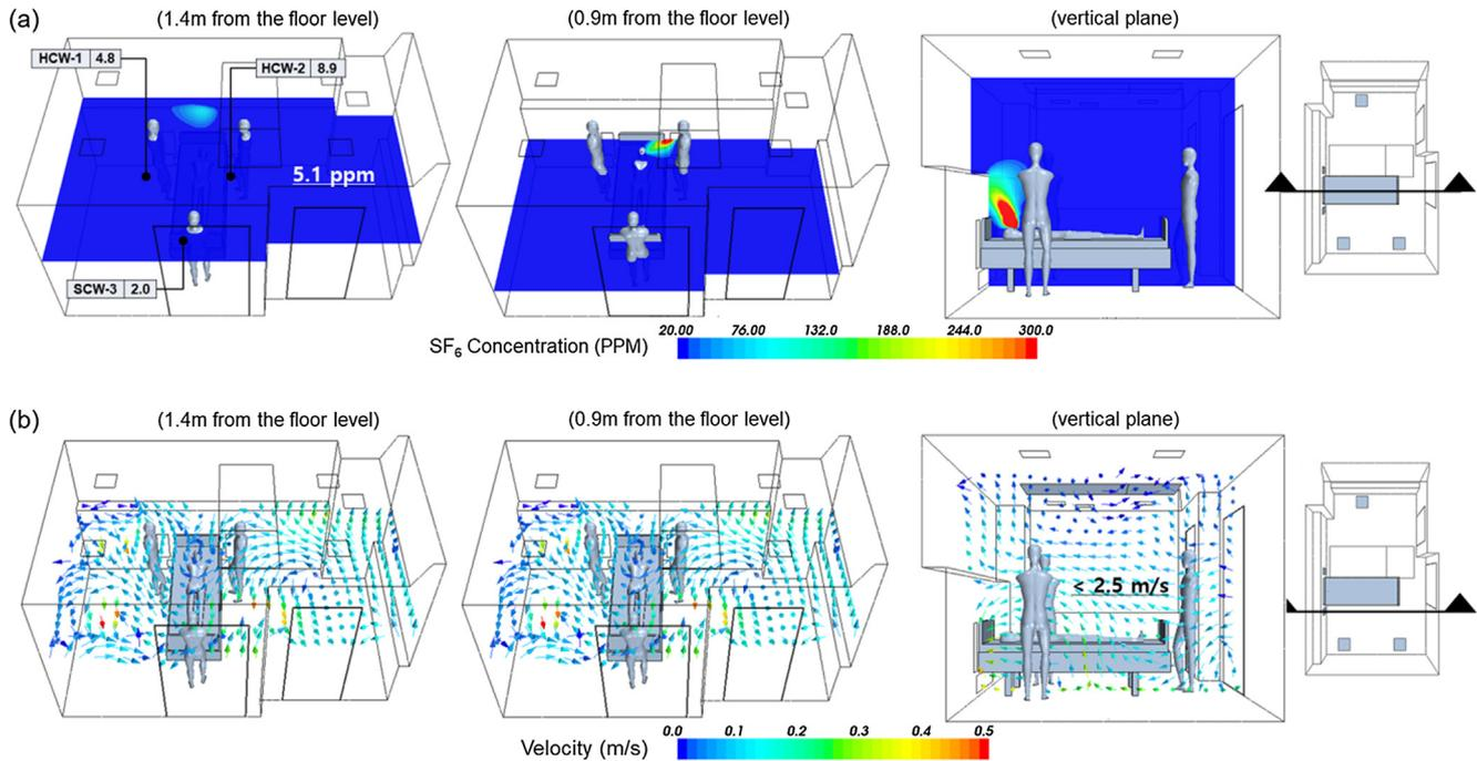
**Fig. 11.** Simulation results of ventilation Case #3 with FFU; (a) concentration profile of SF<sub>6</sub> and (b) velocity vector plot.
