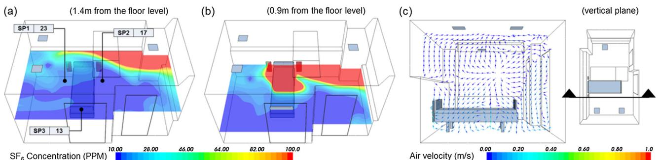
Fig. 8. CFD simulation verification results; (a), (b) concentration profile of SF<sub>6</sub> and (c) velocity vector plot.
