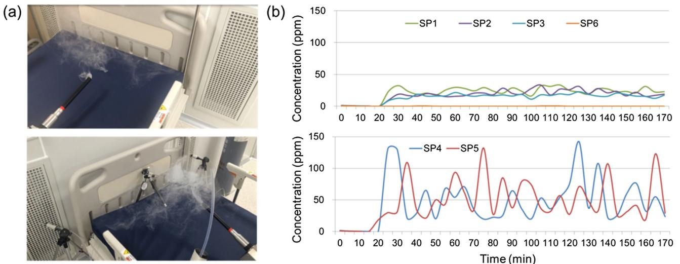
Fig. 7. Measurement results; (a) air flow visualization test in the AIIR and (b) SF<sub>6</sub> concentration profile at the monitoring points.
