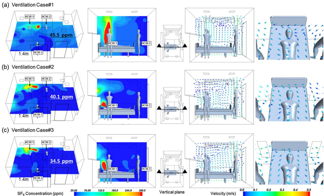
Fig. 5. Simulation results of concentration profile of SF<sub>6</sub> and velocity vector plot; (a) Ventilation Case#1, (b) Ventilation Case#2 and (c) Ventilation Case#3.
