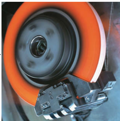
The change from mechanical energy to heat energy is evident in this view of a disk brake.
