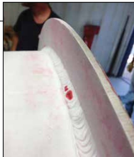
FIGURE 8. The dye penetrant test, an example of NDE, can reveal weld leaks
