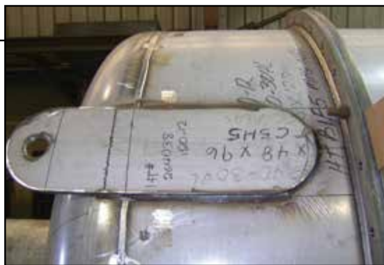
FIGURE 6. Pressure vessel manufacturers transfer information to three or more locations on the piece
