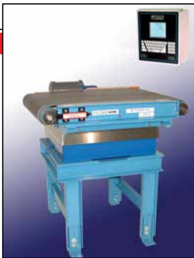
FIGURE 2. Model 4693 filler controller from Thompson Scale offers (among other features) multiple product recipes and optional statistical analysis packages
