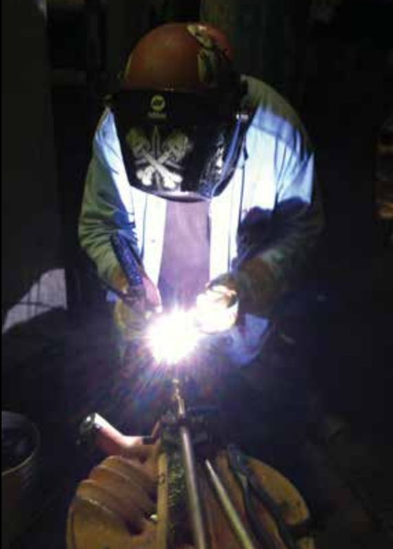
FIGURE 2. Welders must be qualified for each procedure listed in the vessel fabrication drawings
