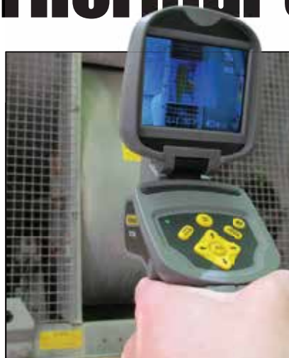
FIGURE 1. Rising temperature is often an indicator of operational problems in many types of machinery. The ability to gather and analyze temperature data in realtime using non-contact options can help operators to pinpoint issues and act accordingly
