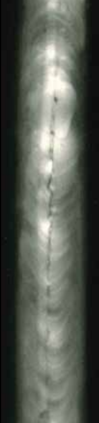
FIGURE 7. Radiographs can reveal flaws not visible in outer appearance
