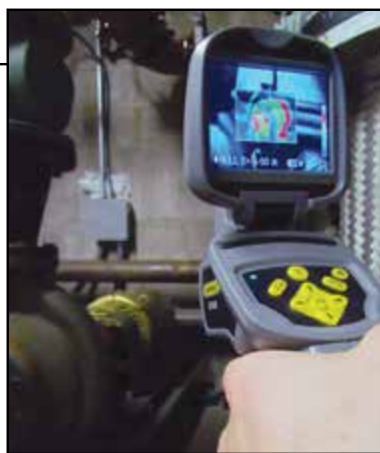
FIGURE 4. Designed with an easy-to-use pistol grip, thermal-imaging cameras are used to diagnose hot spots in machinery systems
