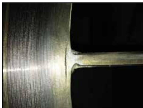
FIGURE 1. Vessel manufacturers need to have a system for identifying nonconformities, such as this scratch in a vessel component
