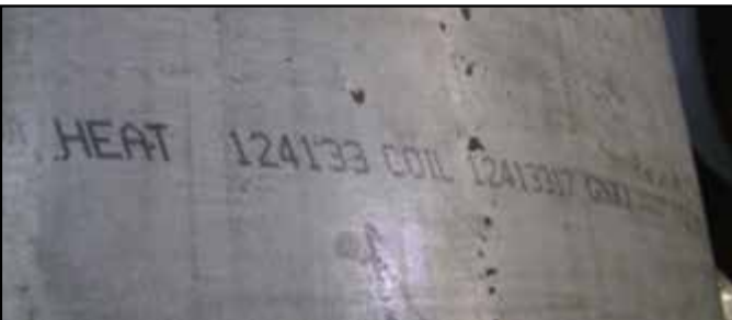
FIGURE 4. Materials to be used for fabricating pressure vessels are inspected to verify compliance with the ASME Boiler and Pressure Vessel Code
