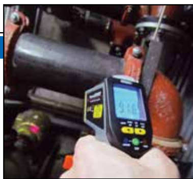
FIGURE 6. Infrared thermometers let users determine the temperature of a specific point on hot or cold surfaces remotely, which is especially useful for inaccessible or hard-to-reach objects or areas. D:S ratio is an important feature to consider when choosing an IRT
