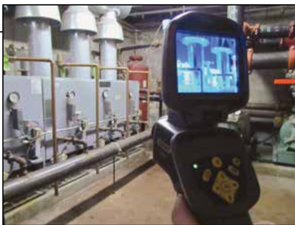
FIGURE 3. Thermal-imaging cameras measure the surface temperature of the objects or areas being analyzed in terms of the amount of infrared (IR) energy that is emitted, transmitted or reflected by the object. The data can then be rendered as still or video images to help operators interpret the result
