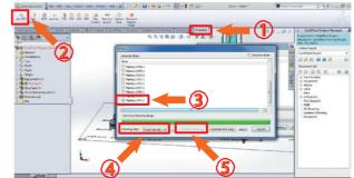
After the generation is finished, there will be a dialog to notify us together with the showing of the output drawing in the item called Isometric Drawing under the Document List as seen here. Now, the drawing has already been generated. We can see the dialog showing status for us to know if there is any error. Then click OK. After that the drawing will be automatically opened for us. Now, SolidWorks has already generated the drawing. Click OK, and then it is time to check the drawing.
