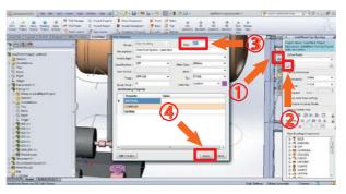
Here, the face of the pump is flange of 8-inch size. Please see that the current value is now 6 inches, so we will change it to 8 inches. After that, select at the Routing Ribbon, and choose Manual Route. We will connect from the flange, so first we will open "Snap to center'. And then snap here and draw the Sketch along X axis for a short distance, and then click and press Escape button. Now we have already got the short piece of pipe.
