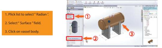
Next, We will input angle value to be 270 degrees, which means that it is located below. And we will set distance to be 200 mm, and Nozzle length to be 150 mm. When finished, click Apply to check it.
