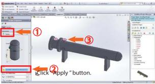
We will input angle parameter to be 90 degrees, distance to be zero -- which is exactly at the datum point, and the Nozzle length to be 150 mm. When done, click Apply.
