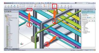
After that, click to be active at SolidPlant Pipe Routing, and we can see that the current active route is line 024. And then go to Routing Ribbon, and click at Jog Route feature.
