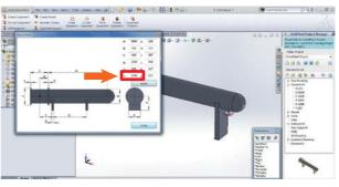
Return to our model. We can see that the heat exchanger now gets taller, and the pipes have adjusted their lengths accordingly. Here, we can notice that the valve has fallen out. This is not a problem, because we can fix it. Make it active by double-clicking at its center line, and make relation it back again. By use mate here at this point, it is fixed, so we will take it out.
