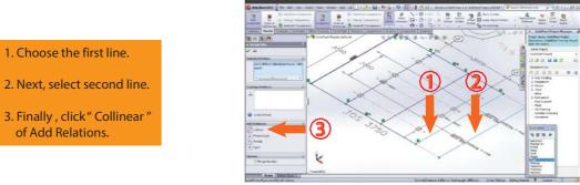
In the same way, I want to change this grid line to be on this line of the plot plan. We can also do that by adding relation to be Colinear. It will appear as required.
