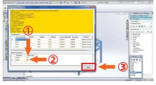
Instantly, a dialog will appear. Please notice the names of Structural Member, which are shown as name and order of part list. The numbers are run for all parts. As from below, total length of each type of shape is also shown. The whole length of each shape type will appear here. Moreover, we can export data as an Excel file. To do that, click Export to Excel.
