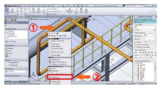
Next, click at the required positions to be the first point and the second point. Initially, we will click to define the position, but we will not set the distance at this moment. After that, press Escape button to break the pipe. Please notice that now it has already divided the pipe into 3 parts - one, two, and three. Zoom to closely see it. Here we can select the middle part by clicking at its center line. After that, go to Routing Ribbon to select the feature of Change Size by clicking it.
