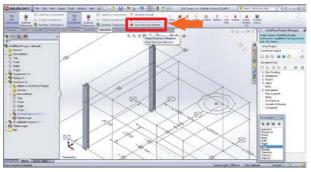
The concept of beam placing is to make a point-to-point sketch, starting from this point and drawing to this point.
