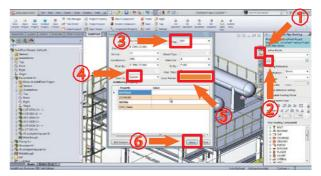
Go to Routing Ribbon, and select the Manual Route feature. After that, open Snap to Center. Zoom-in at this nozzle, select at the edge, and select center. Next, lock the axis to be along Z axis by press Tab button on the keyboard. After that, continue to draw toward the side along Y axis. And then, we will draw further to the left along X axis, and click. Next, draw up along Z axis. When done, press Escape to generate the pipe.
