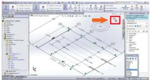
After that, we will input data for levels. We can do that by editing the grid frame again. Go to Structure Ribbon, and then click at 3D grid. And click the button of Structure 3D Grid.
