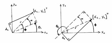
This results in a total of two solutions. Finally, we project the first three links of the manipulator onto the  $x_0 - y_0$  plane to find solutions for waist angle  $\theta_1$ .
