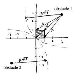
– Assume the robot has three degrees of freedom, and thus three "joint variables"  $q = \{x, y, \theta\}$ . The robot is able to translate  $\{x, y\}$  (think of this as two prismatic joints) and rotate  $\{\theta\}$  (think of this as a single revolute joint).
