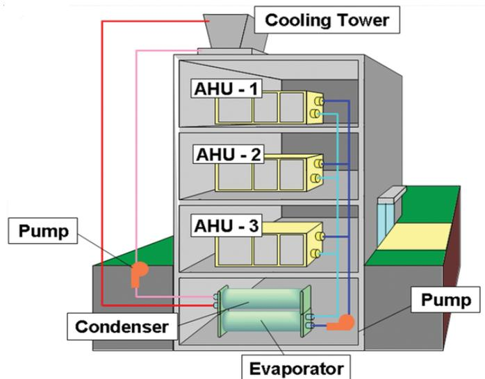
Figure 1 Chilled Water System Overview
