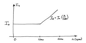
part (b): In this case, the torque will remain constant as the speed is increased to 1200 r/min. However, as the field flux drops to increase the speed above 1200 r/min, it is not possible to increase the armature current as the field flux is reduced to increase the speed above 1200 r/min and hence the torque track the field flux and will decrease in inverse proportion to the change in speed above 1200 r/min.
