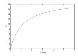
part (c): During this time, starting at time t=5.71 msec, v(t)=-75 V and  $L_(t)=26.0\times 10^{-3}-3.76(t-5.71\times 10^{-3})$ . Thus
