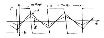
$$E_{\text{max}} = 4fNA_{\text{c}}B_{\text{peak}} = 345 \text{ V}$$
