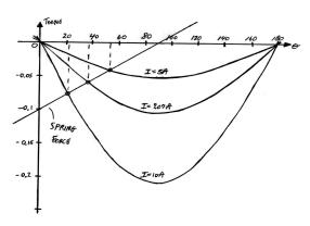
part (e): The curve of spring force versus angle is plotted as a straight line on the plot of part (d). The intersection with each curve of magnetic force versus angle gives the equilibrium angle for that value of current. For greater accuracy, MATLAB can be used to search for the equilibrium points. The results of a MATLAB analysis give:
