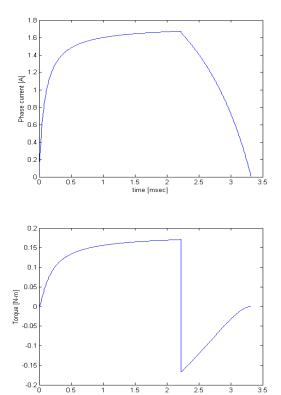
The integral under the torque curve is  $2.38 \times 10^{-4}$  N·m·sec while the positive torque integral is 3.29 N·m·sec. Thus there is a 25.7% reduction in torque due to negative torque production during the current-decay period.
