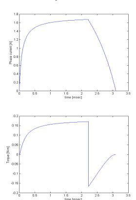
The integral under the torque curve is  $2.59 \times 10^{-4}$  N·m·sec while the positive torque integral is 3.20 N·m·sec. Thus there is a 19.0% reduction in torque due to negative torque production during the current-decay period.
