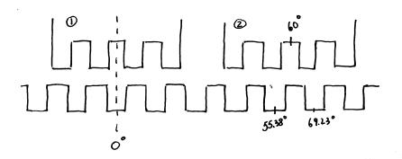
From the figure, we see that if phase 1 is turned off and phase 2 is energized, the rotor will rotate 4.61° degrees to the right (clockwise) to align with the phase-2 pole. Similarly, if phase 3 is excited after phase 1 is turned off, the rotor will rotate 4.61° degrees to the left (counterclockwise).
