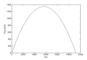
An iterative MATLAB scripts can easily find the two desired operating points: 2761 r/min for which the efficiency is 24.3% and 8473 r/min for which the efficiency is 72.8%.
