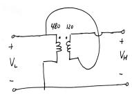
part (b): The rated current of the high voltage terminal is equal to that of the 120-V winding,  $I_{\rm rated}=10^4/120=83.3$  A. Hence the kVA rating of the transformer is  $600\times83.3=50$  kVA.
