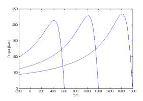
part (b): The same MATLAB script can be used to iteratively find the drive frequency for which  $s_{\text{maxT}} = 1.0$ . The result is a drive frequency of 5.44 Hz and a torque of 151 N·m.
