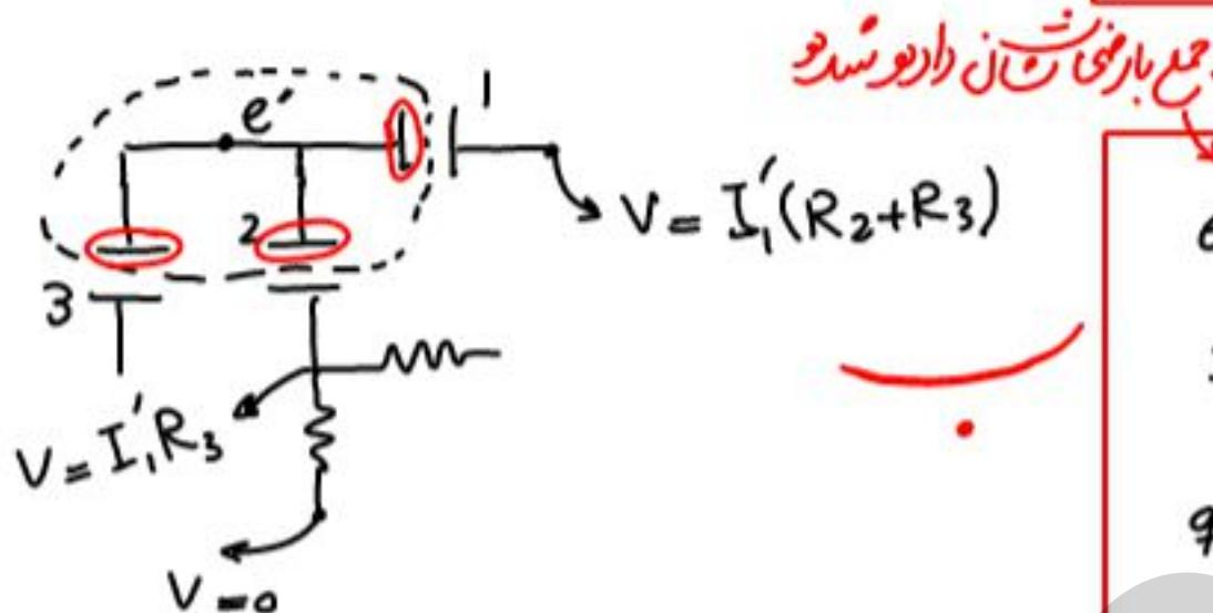
$$e' C_3 + (e' - I' R_3) C_2 + (e' - I' R_2 - I' R_3) C_1 = q_3$$
