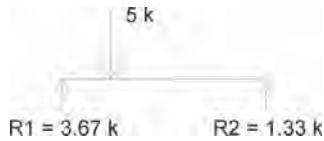
FIGURE 1.21 Simple beam resultant force solution.
