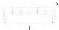
FIGURE 6.3 Typical loading diagram for lagging.
