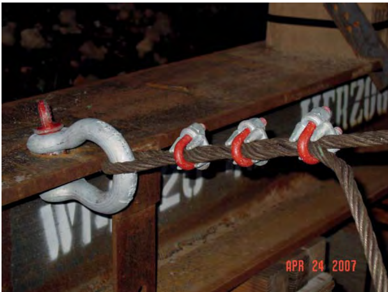
FIGURE 11.18 Wire rope connection with clips and thimbles.
