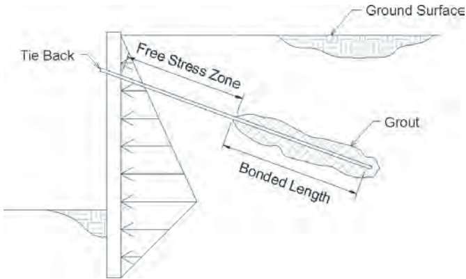
FIGURE 6.24 Bonded and unbonded zones of a tieback.
