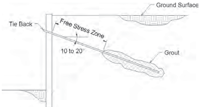
FIGURE 6.22 Soil anchor embedded behind failure plane.
