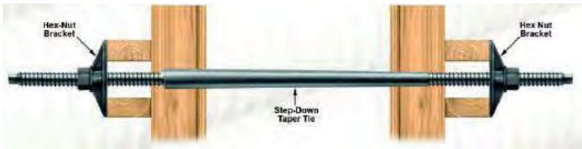
FIGURE 9.14 Taper tie cross section.
