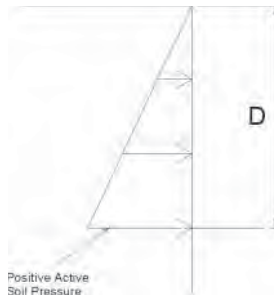
FIGURE 5.8 Active soil pressure diagram.
