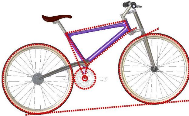
When combined with in-context techniques, assembly layout sketches can help to determine the shape of parts, or the location, size, or shape of features within the parts. You also can use layout sketches to mate assembly components to far more robust and dependable mates, rather than mating part to part. The sketch shown in Figure 13.8 is used for both of these techniques. The shape of the frame and the major pivot points are established in the 2D sketch. The wheels also are mated to the sketch.
