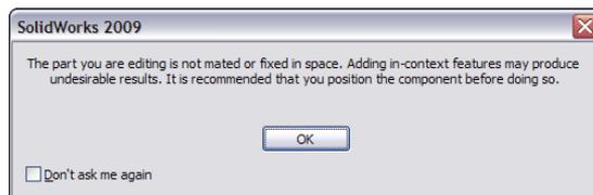
This message should remind you that in-context features should be used only on parts that are fully positioned in the assembly.
