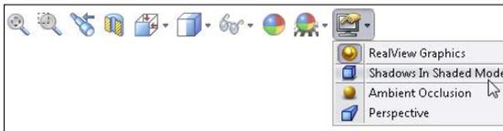
When you are using Shadows in shaded mode, you can take advantage of a special scene called Ambient Occlusion. With this combination, the SolidWorks model can throw shadows on itself, and holes in the model appear in shadow. It gives some of the effect of a rendering, but it is just the RealView display.
