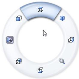
It may take a little time for you to get used to the interface. It works best when you understand what the commands are before you use them, so you can invoke the Top View command in a single motion. It does not work well if you have to initiate the interface with a very short RMB drag and then drag again to select the command. For this reason, it might
