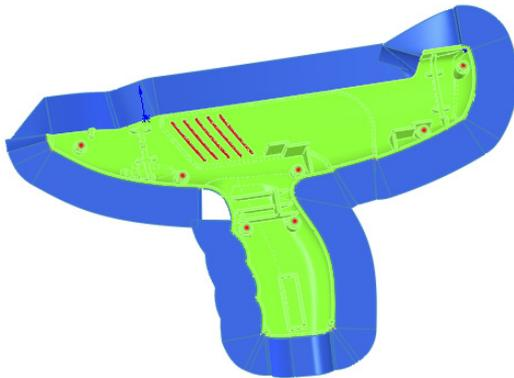
From this, you can learn that the SolidWorks Mold Tools are not reliable for concave parting lines or non-planar parting lines. Flat parting line disks and boxes work well. Beyond that, you should expect to do some manual surface modeling.
