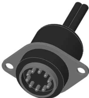
There's nothing special about this part. It's modeled in SolidWorks using standard features, and there are no configurations or special features. It could have been downloaded from 3D Content Central. It represents an electrical connector that may be mounted in a sheet metal electrical enclosure.
