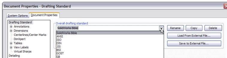
The drafting standard file type has the extension of \*.sldstd. If someone else has sent you a standard file, you can read it in to your drawing using the settings shown on the right of Figure 24.2 and assign it as the active standard; your drawing will assume all the customized properties.
