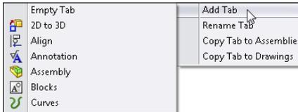
To add individual buttons, first find the button you want to add in the Customize dialog box by choosing Tools ⇨ Customize. Click the Commands tab in the Customize dialog box, and then switch the CommandManager to the tab you want to add the button to, and drag the button from the Customize dialog box to the CommandManager. You can remove buttons from the CommandManager by dragging them into the blank graphics window area.
