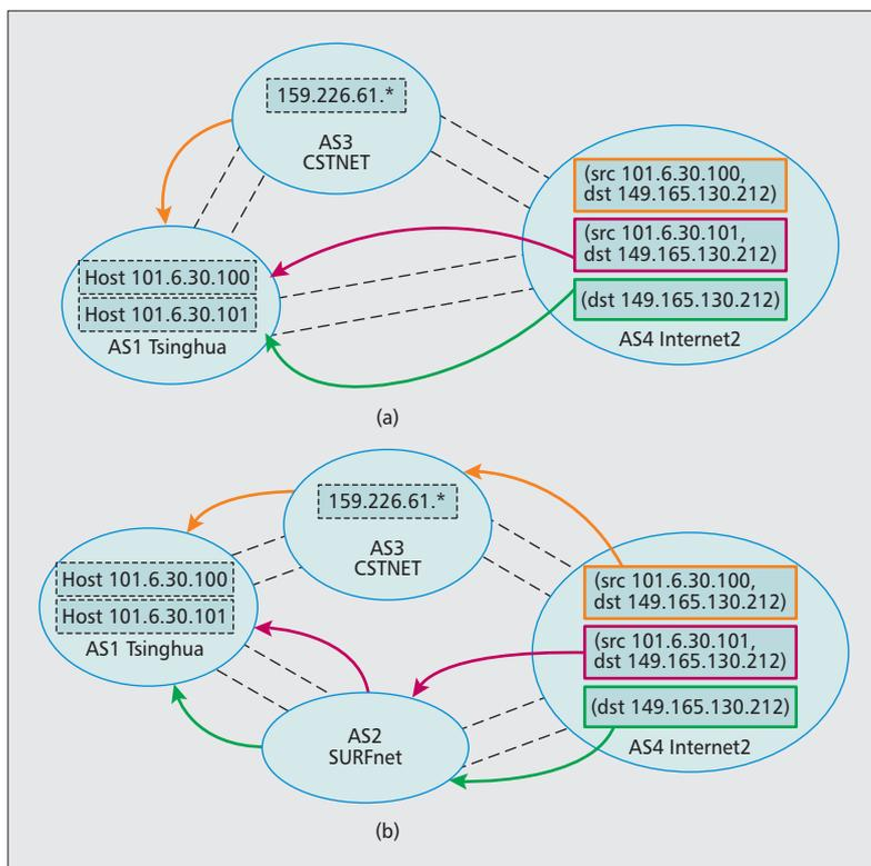
**Figure 4.** A concept illustration of source address based multipath routing.
