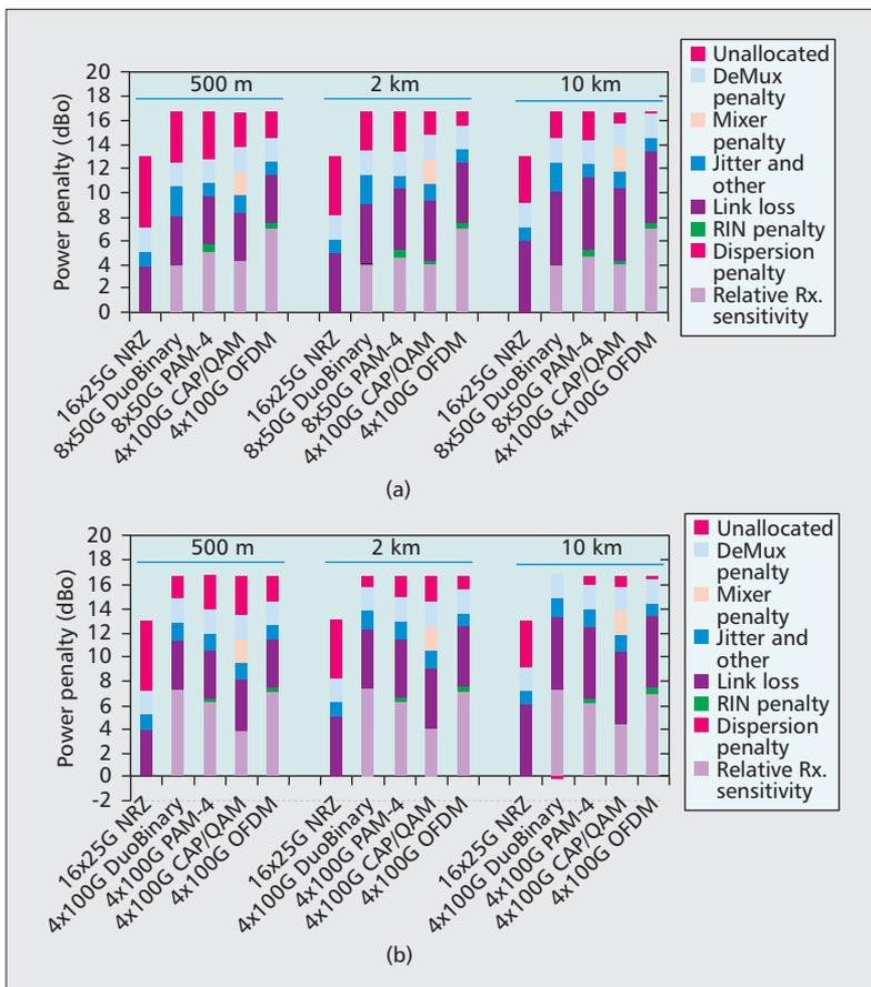
**Figure 5.** Link optical power penalties for various 400 GbE links using different modulation formats under: a) DML case; b) EML case.
