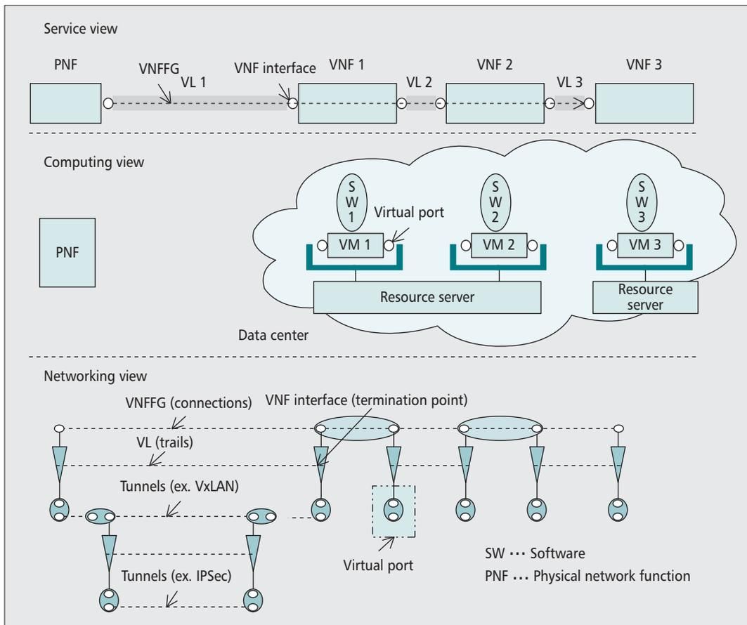
Figure 4. Function modeling for an example virtual network.
