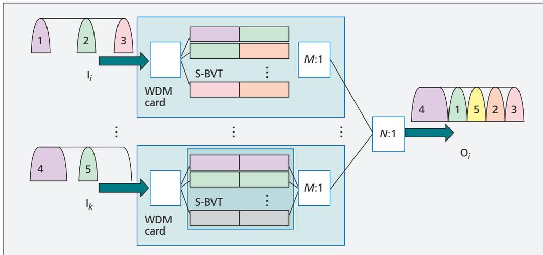
**Figure 5.** Exploitation of SERANO properties for defragmentation.
