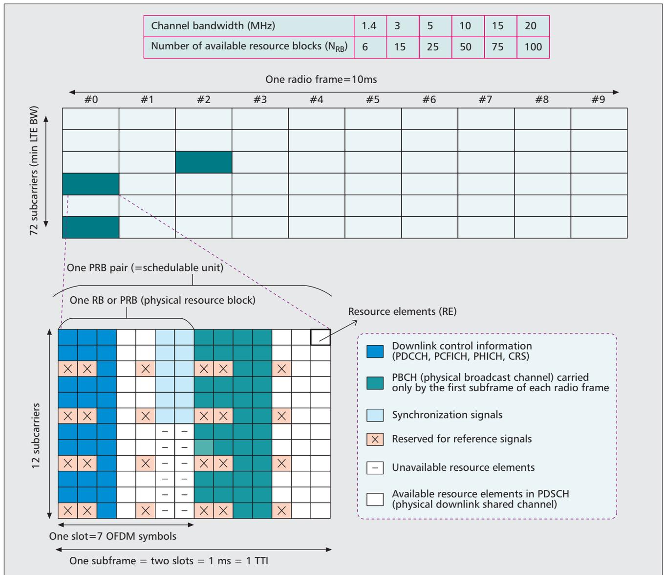
**Figure 1.** Downlink radio frame structure with four antenna ports in LTE/LTE-Advanced (reproduced from 3GPP specifications [14]).
