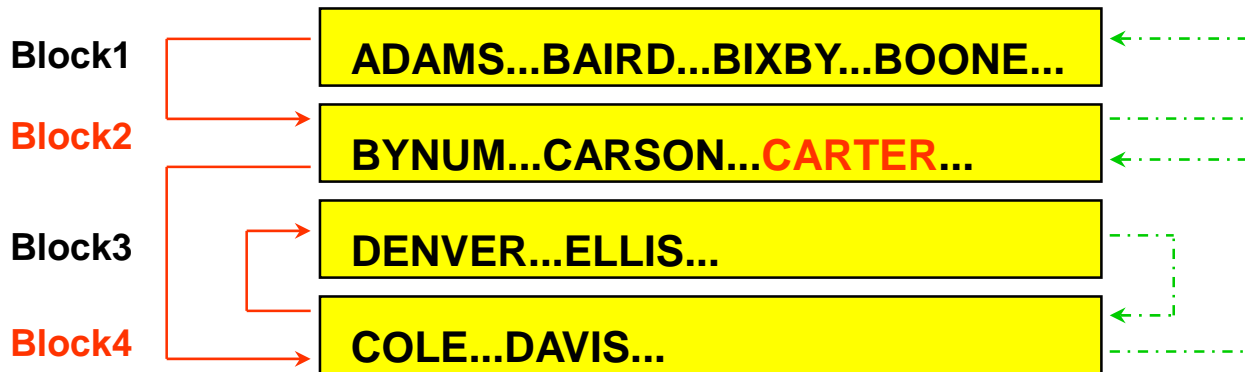
(b) Sequence set after insertion of CARTER record - block 2 splits , and the contents are divided between blocks 2 and 4
