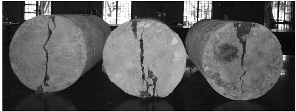
Fig. 9 Splitting failure mode of the E-plastic concrete specimen after ultimate load
