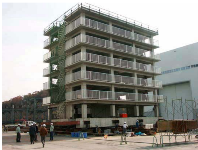
Figure 7. Six-story RC frame model prepared for test on Miki Table
