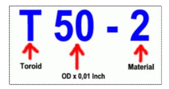
T means toroid (ring core). The following figures are representing the outer diameter in 0,01 inch. The figure(s) after the dash indicating the mixture of material and therewith the usable frequency range, indicated by the color of the core. Through both list fields
