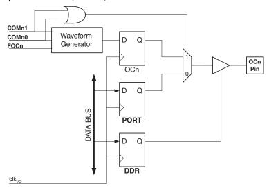
Figure 56. Compare Match Output Unit, Schematic
