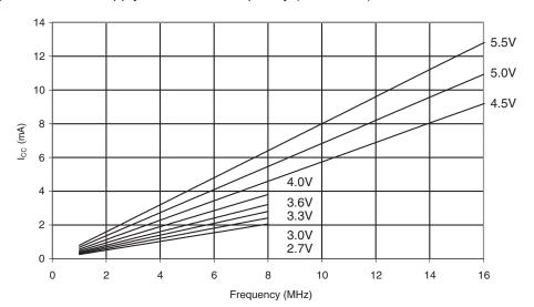
Figure 155. Idle Supply Current vs. Frequency (1 - 16MHz)
