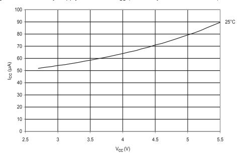
Figure 167. Standby Supply Current vs. V<sub>CC</sub> (2MHz Crystal, WDT Disabled)
