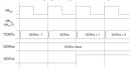
Figure 50 shows the same timing data, but with the prescaler enabled.
