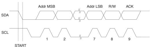
Figure 79. Address Packet Format
