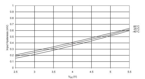
Figure 181. I/O Pin Input Hysteresis vs.  $V_{CC}$
