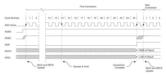
Figure 102. ADC Timing Diagram, Single Conversion
