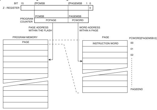
Figure 126. Addressing the Flash during SPM<sup>(1)</sup>
