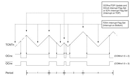
Figure 47. Phase Correct PWM Mode, Timing Diagram
