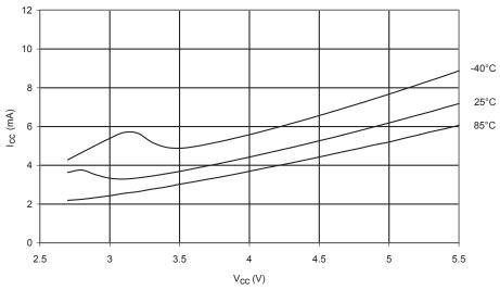
Current Consumption in Reset and Reset Pulsewidth
