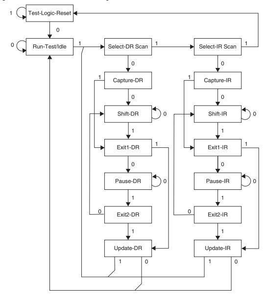
Figure 113. TAP Controller State Diagram
