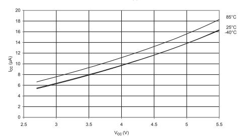
Figure 161. Power-down Supply Current vs.  $V_{\text{CC}}$  (Watchdog Timer Enabled)
