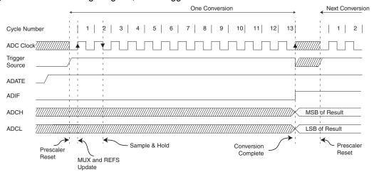
Figure 103. ADC Timing Diagram, Auto Triggered Conversion
