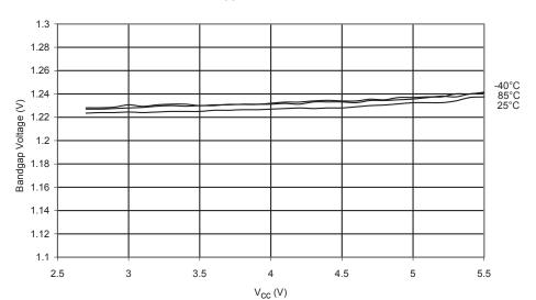
Figure 187. Bandgap Voltage vs.  $V_{CC}$
