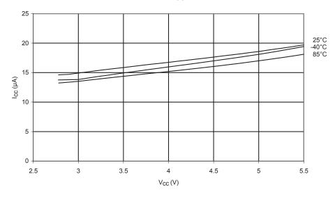
Figure 202. ADC Current vs.  $V_{CC}$  (AREF = AVCC)
