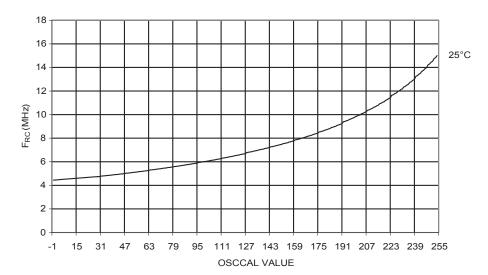
Figure 191. Calibrated 8MHz RC Oscillator Frequency vs. Osccal Value
