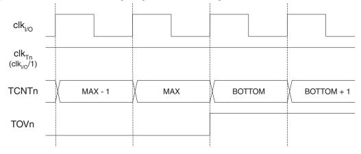
Figure 61 shows the same timing data, but with the prescaler enabled.
