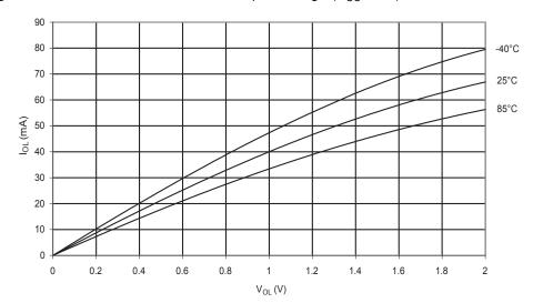
**Figure 177.** I/O Pin Sink Current vs. Output Voltage  $(V_{CC} = 5V)$
