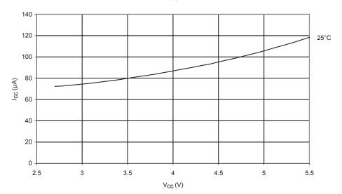
Figure 165. Standby Supply Current vs.  $V_{CC}$  (4MHz Crystal, WDT Disabled)
