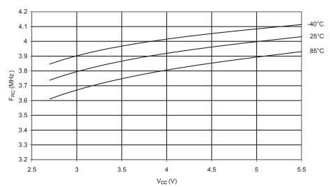
Figure 193. Calibrated 4MHz RC Oscillator Frequency vs.  $V_{\rm CC}$
