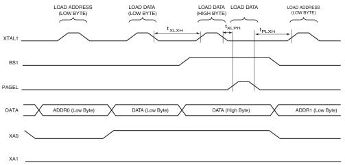
Note: 1. The timing requirements shown in Figure 133 (that is, t<sub>DVXH</sub>, t<sub>XHXL</sub>, and t<sub>XLDX</sub>) also apply to loading operation.
