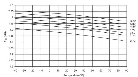
Figure 195. Calibrated 2MHz RC Oscillator Frequency vs. Temperature
