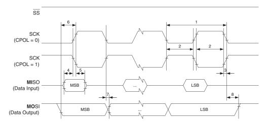
Figure 146. SPI Interface Timing Requirements (Master Mode)
