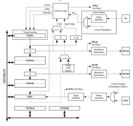
Figure 40. 16-bit Timer/Counter Block Diagram<sup>(1)</sup>
