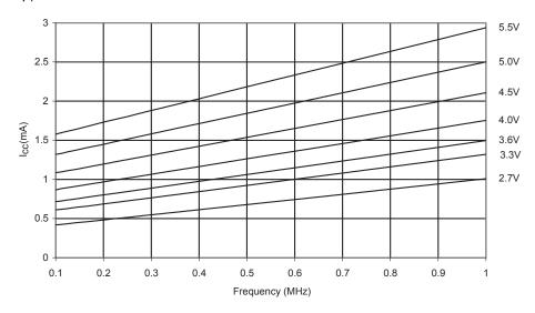
**Figure 207.** Reset Supply Current vs.  $V_{CC}$  (1 - 16MHz, Excluding Current Through The Reset Pull-up)
