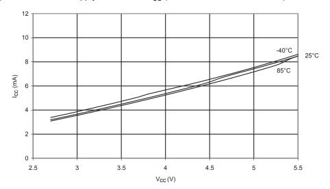
Figure 151. Active Supply Current vs.  $V_{\text{CC}}$  (Internal RC Oscillator, 4MHz)
