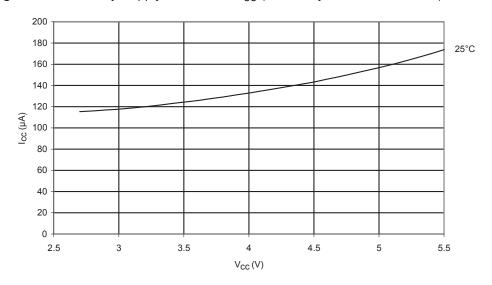
Figure 164. Standby Supply Current vs.  $V_{CC}$  (6MHz Resonator, WDT Disabled)
