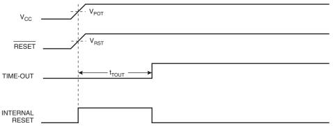
Figure 17. MCU Start-up, RESET Extended Externally
