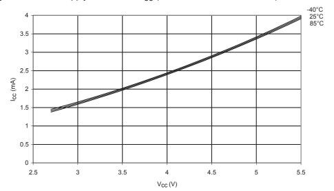
Figure 157. Idle Supply Current vs.  $V_{\text{CC}}$  (Internal RC Oscillator, 4MHz)
