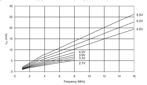
Figure 149. Active Supply Current vs. Frequency (1 - 16MHz)
