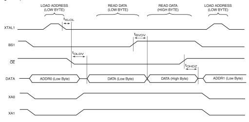
Note: 1. The timing requirements shown in Figure 133 (that is,  $t_{DVXH}$ ,  $t_{XHXL}$ , and  $t_{XLDX}$ ) also apply to reading operation.
