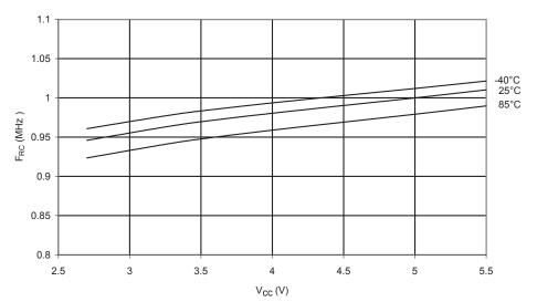
Figure 199. Calibrated 1MHz RC Oscillator Frequency vs.  $V_{\rm CC}$
