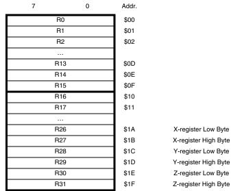
General Purpose Working Registers X-register High Byte Y-register High Byte
