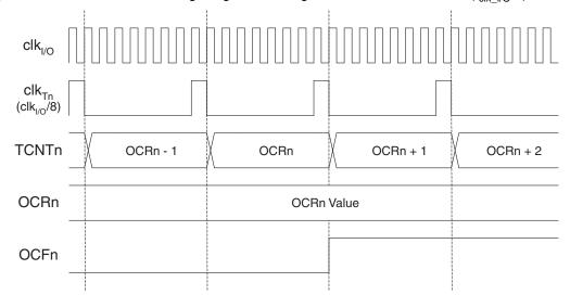
Figure 37 shows the setting of OCF0 and the clearing of TCNT0 in CTC mode.
