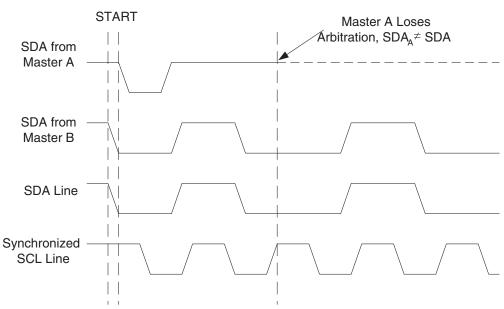
Figure 83. Arbitration between Two Masters
