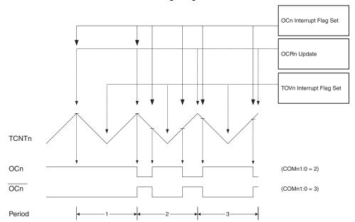
Figure 59. Phase Correct PWM Mode, Timing Diagram
