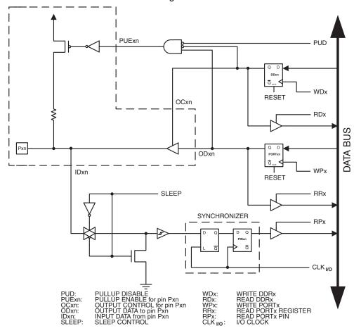
Figure 117. General Port Pin Schematic Diagram<sup>(1)</sup>
