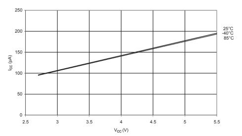
Figure 203. AREF External Reference Current vs.  $V_{\text{CC}}$
