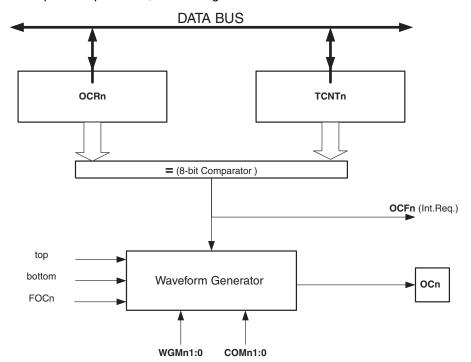
Figure 29. Output Compare Unit, Block Diagram
