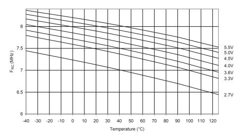
Figure 189. Calibrated 8MHz RC Oscillator Frequency vs. Temperature
