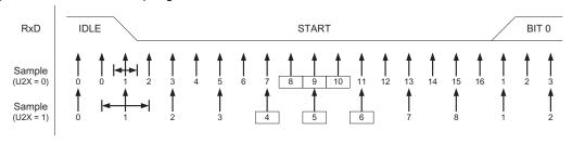
When the clock recovery logic detects a high (idle) to low (start) transition on the RxD line, the start bit detection sequence is initiated. Let sample 1 denote the first zero-sample as shown in the figure. The clock recovery logic then uses samples 8, 9, and 10 for Normal mode, and samples 4, 5, and 6 for Double Speed mode (indicated with sample numbers inside boxes on the
