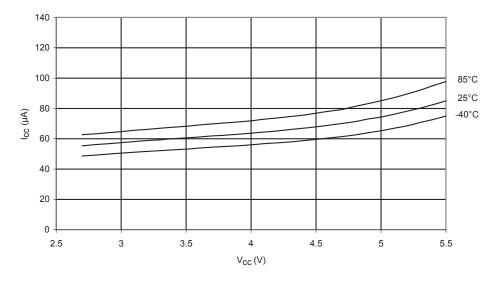
Figure 205. Programming Current vs.  $V_{\text{CC}}$
