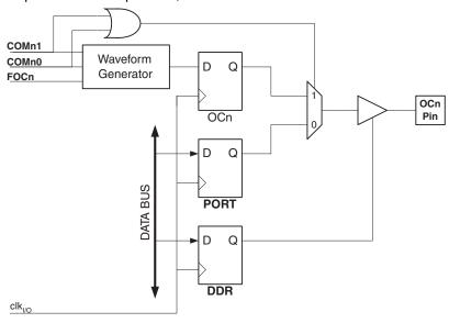
Figure 30. Compare Match Output Unit, Schematic
