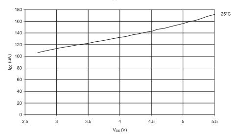
Figure 153. Active Supply Current vs. V<sub>CC</sub> (External Oscillator, 32kHz)
