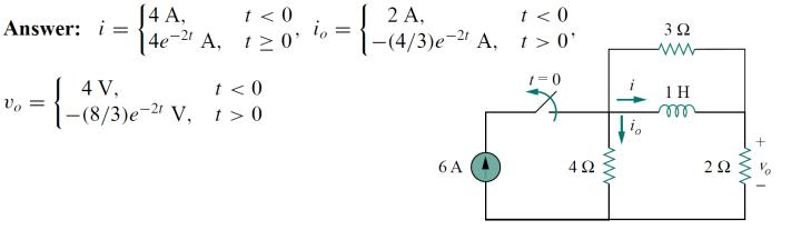
6- The switch in Fig. 7.47 is closed at t = 0. Find i(t) and v(t) for all time. Note that u(-t) = 1 for t < 0 and 0 for t > 0. Also, u(-t) = 1 - u(t).
