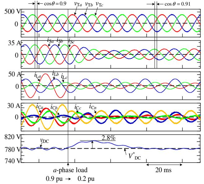
Fig. 5. Simulation waveforms using the proposed reactive power control strategy with heavy-load to light-load variation (power factor is set to 0.9).
