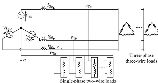
Fig. 1. Three-phase four-wire distribution systems.
