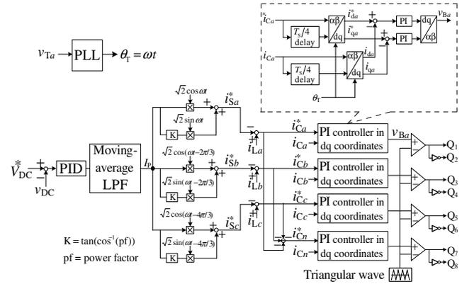
Fig. 3. Proposed reactive power control strategy for the active load balancer.
