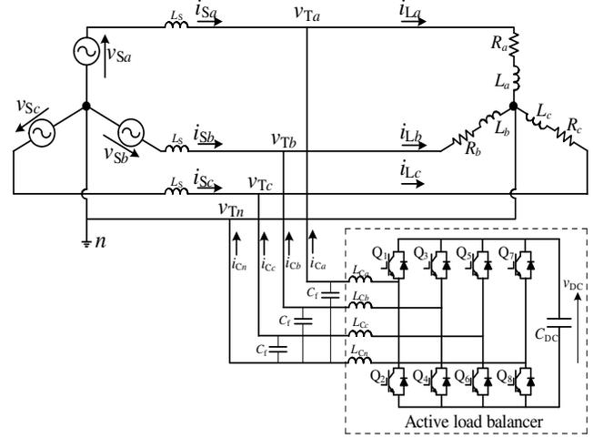
Fig. 2. Power circuit diagram of the proposed active load balancer.
