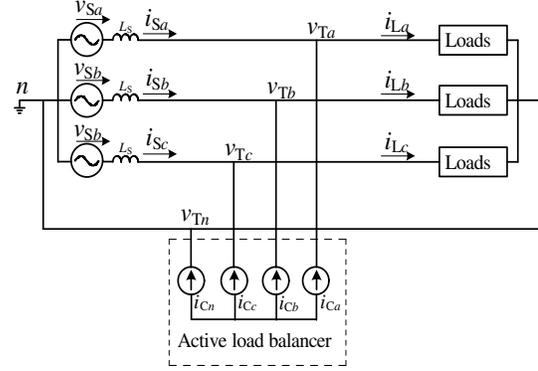
Fig. 10. Equivalent circuit of the ALB in three-phase four-wire distribution systems.
