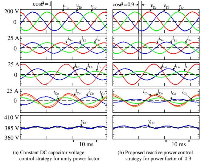
Fig. 11. Comparison of experimental waveforms using two control strategies for the ALB.
