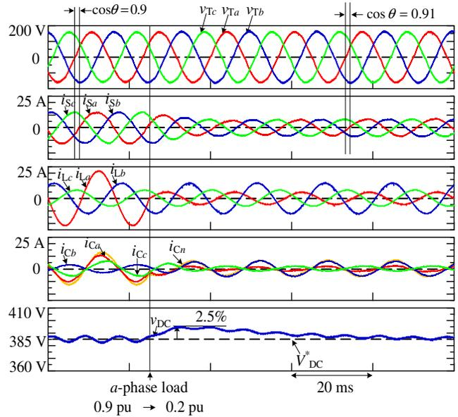
Fig. 8. Experimental results of the proposed reactive power control strategy with heavy-load to light-load variation (power factor is set to 0.9).
