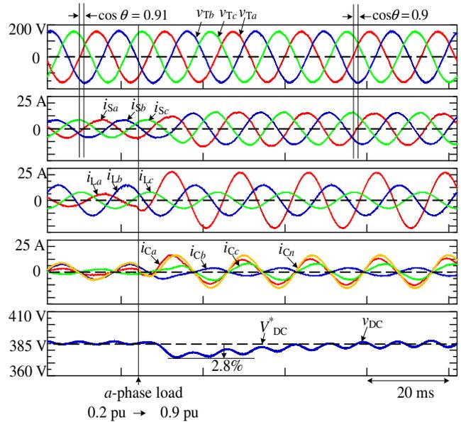
Fig. 9. Experimental results of the proposed reactive power control strategy with light-load to heavy-load variation (power factor is set to 0.9).
