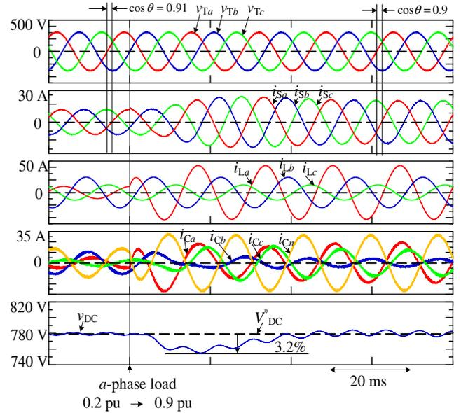
Fig. 6. Simulation waveforms using the proposed reactive power control strategy with light-load to heavy-load variation (power factor is set to 0.9).
