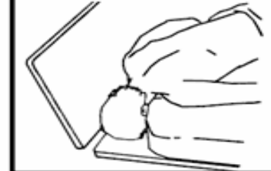
Zone 7 - Entrapment between head or foot board and mattress
