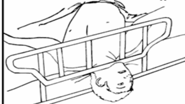
Zone 2 - Entrapment between top of compressed mattress to bottom of rail, between rail and supports
