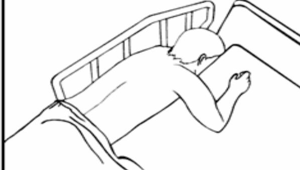
Zone 3 - Entrapment in horizontal space between rail and mattress
