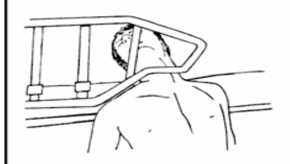
Zone 4 - Entrapment between top of compressed mattress and bottom of rail at end of rail
