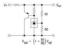
Figure 19. High Current Shunt Regulator
