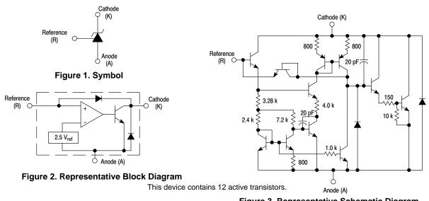
Figure 3. Representative Schematic Diagram Component values are nominal
