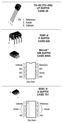
This is an internally modified SOIC–8 package. Pins 2, 3, 6 and 7 are electrically common to the die attach flag. This internal lead frame modification increases power dissipation capability when appropriately mounted on a printed circuit board. This modified package conforms to all external dimensions of the standard SOIC–8 package.
