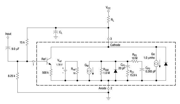
Figure 31. Simplified TL431 Device Model
