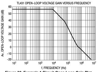
**Figure 32. Example 1 Circuit Open Loop Gain Plot** Example 2.
