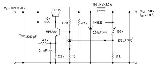
Figure 30. High Efficiency Step–Down Switching Converter
