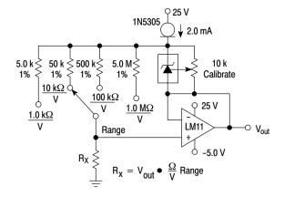
Figure 28. Linear Ohmmeter
