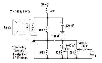
Figure 29. Simple 400 mW Phono Amplifier
