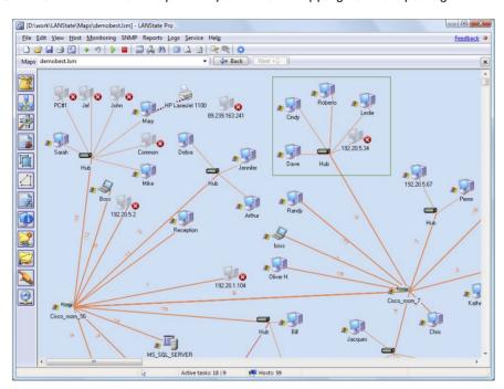
FIGURE 5.7 A network map built by a network-mapping software package
