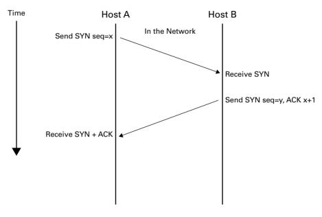
FIGURE 5.2 Half-open scan against closed and open ports
