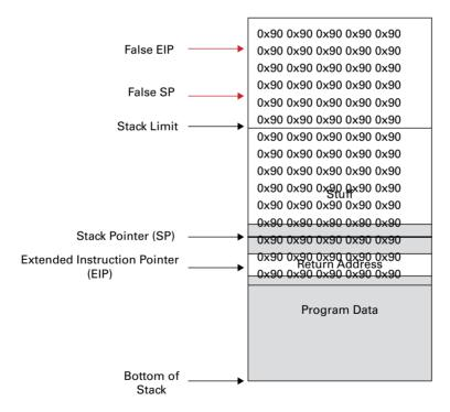
Figure 11.2 deserves just a bit more explanation, as it may look a little confusing at this point. Let's take it one piece at a time. Underlying the "0x90" block (which will be discussed in "NOP Sled" in a moment) is the basic program stack from Figure 11.1. Remem-
