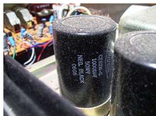
Figure 2. 41 A reservoir capacitor in an amplifier
