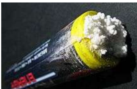
Figure 6.36 A leaked alkaline battery
