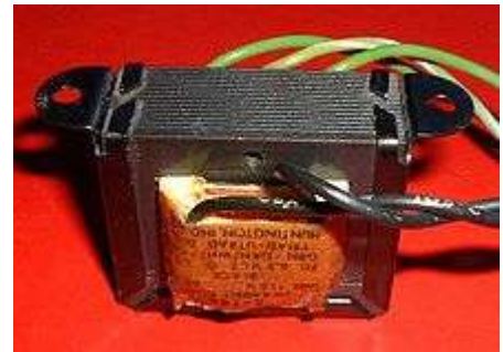
Figure 2. 49 A transformer with laminated steel core
