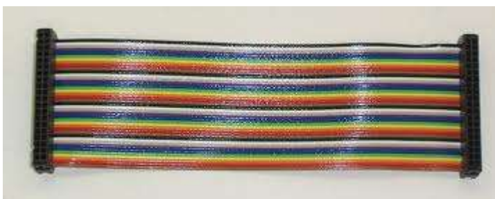
Figure 2. 20 The ribbon cable for connecting computer peripherals
