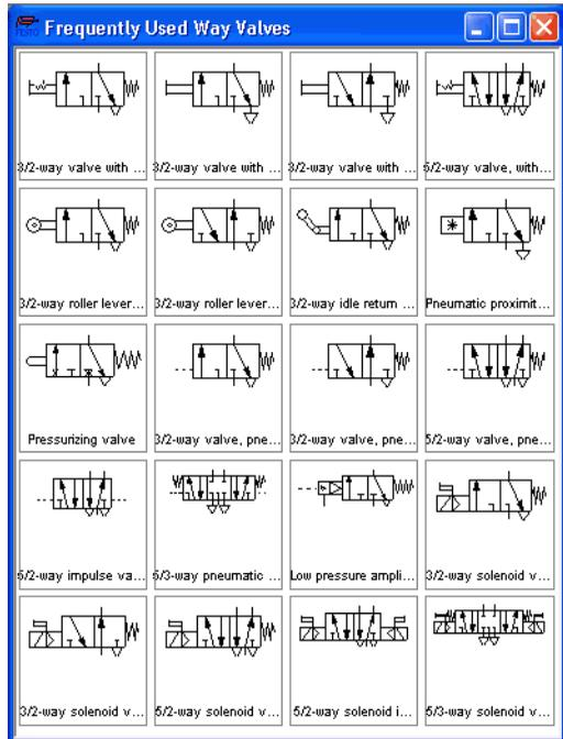
In contrast to the FluidSIM standard libraries both the arrangement and the contents of such user-defined libraries can be defined, by means of operations that add and delete components.
