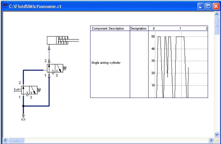
Note that several state diagrams can be used in the same circuit; however, several components may also share the same state diagram. A component is added by simply dropping it onto the state diagram. If a component is dropped a second time on the diagram, it will be removed from there. State quantities of the following components can be recorded and displayed in the state diagram:
