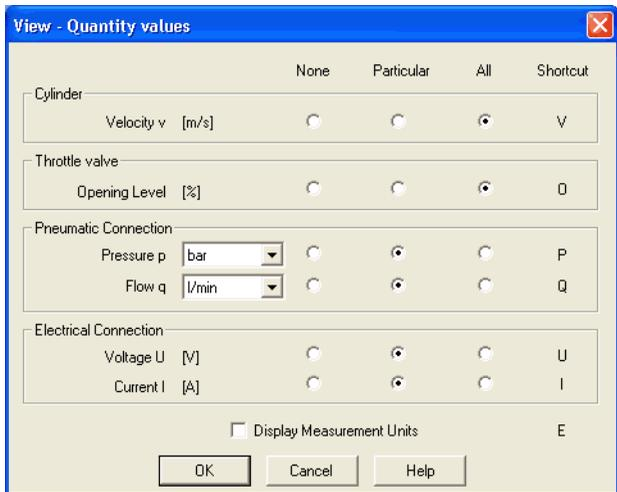
For each of the listed quantities (“Velocity”, “Pressure”, ...) a display mode can be chosen.
