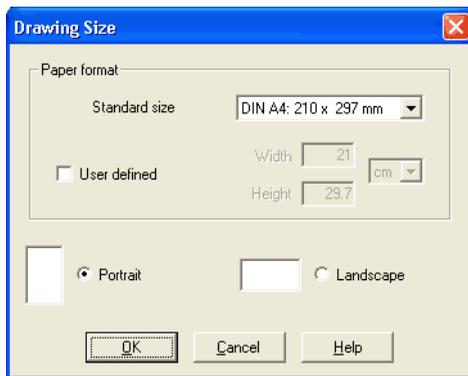
The size and the orientation of the paper can be set here. If the drawing size exceeds the paper size of your printer, the total area of several smaller papers can be tiled with the drawing.
