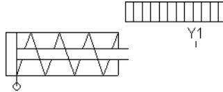
As a consequence, the cylinder will activate the switch or the valve labeled "Y1" if its piston has traveled by 35 mm. To define a label in the electrical circuit double click on the respective component; to define a label at a mechanical actuator of a valve double click the respective "connection" of the valve.
