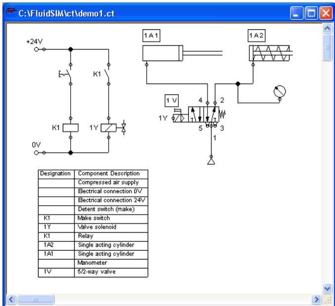
The screenshot displays the FluidSIM software window titled "C:\FluidSIM\ct\demo1.ct". The main area shows a circuit diagram with a +24V supply, a 0V ground, a switch K1, a valve solenoid 1Y, a relay K1, a manometer, and two cylinders 1A1 and 1A2. A 5/2-way valve 1V is also present. The parts list table at the bottom provides the following details:
