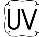
FIG. AR-401.1 OFFICIAL SYMBOL FOR STAMP TO DENOTE THE AMERICAN SOCIETY OF MECHANICAL ENGINEERS' STANDARD
