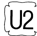
FIG. AS-100.1 OFFICIAL SYMBOL FOR STAMP TO DENOTE THE AMERICAN SOCIETY OF MECHANICAL ENGINEERS’ STANDARD
