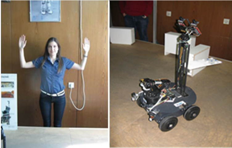
Fig. 15 Gesture command for mobile robot
