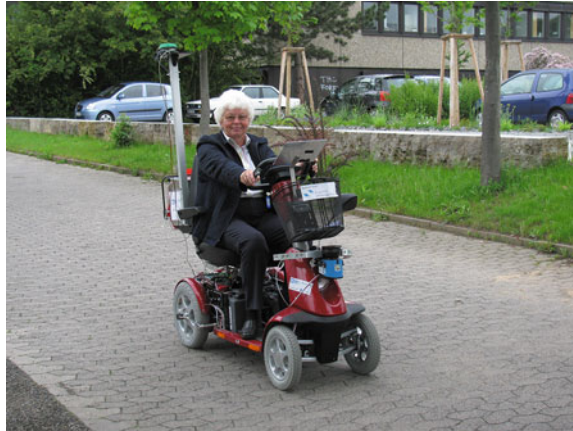
Fig. 1 The mobility scooter Trophy 4W with all hardware extensions during a test run with a member of the senior committee
