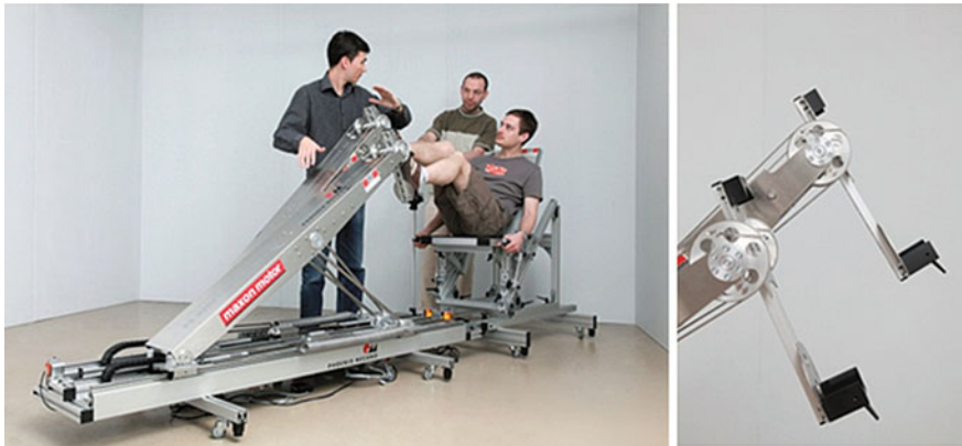
Fig. 3 The Lambda parallel robot for lower limb mobilization developed by LSRO
