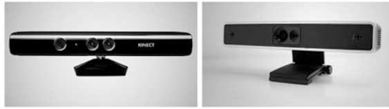
Fig. 1 Sample 3D sensors for indoor applications: left Microsoft Kinect for Windows (Microsoft Corporation 2013), right Softkinetic DepthSense 311 (SoftKinetic 2013)
