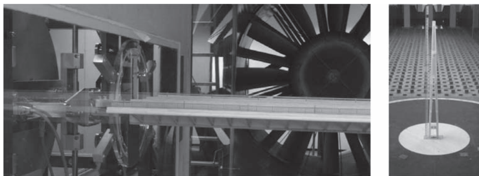
Figure 5. Wind tunnel test at section model of superstructure and a full tower model.
