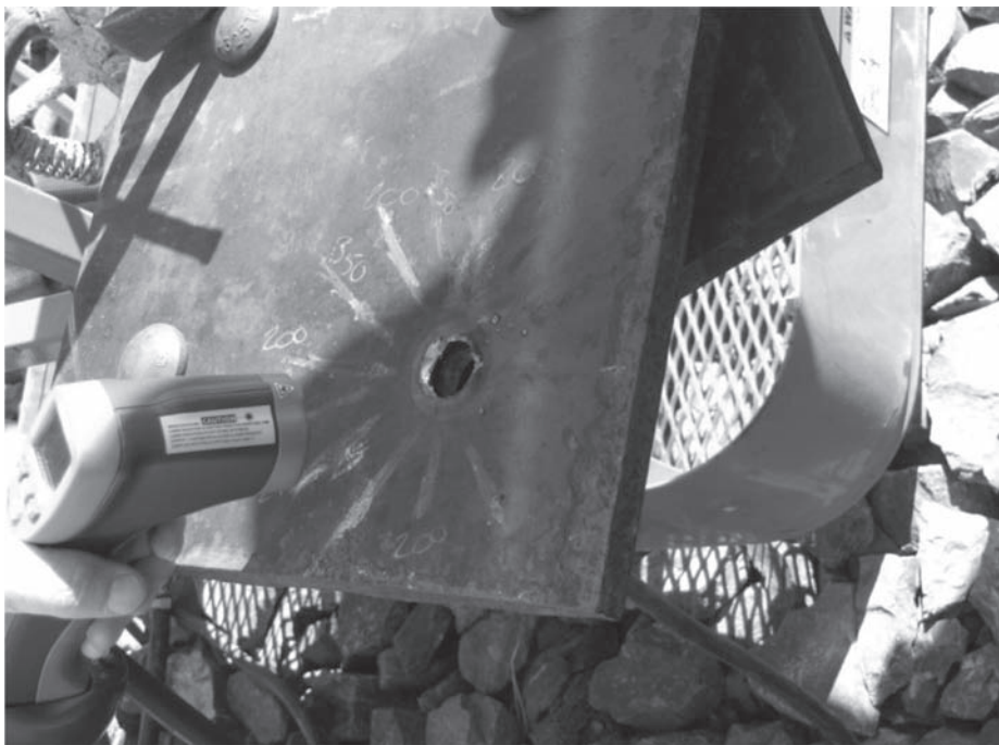
Figure 5. Test specimen plate immediately after air-arc bolt removal.
