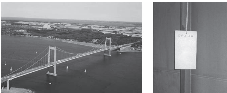
Figure 4. Little Belt Suspension Bridge and untreated steel plate in bridge girder.
