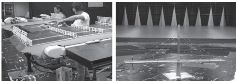
Figure 7. Wind tunnel testing: a) confirmatory deck section. b) balanced cantilever from central tower.
