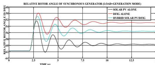
Fig 6: Rotor angle comparison between Solar PV,DFIG and Hybrid SOLAR PV/DFIG (Load=Generation mode)
