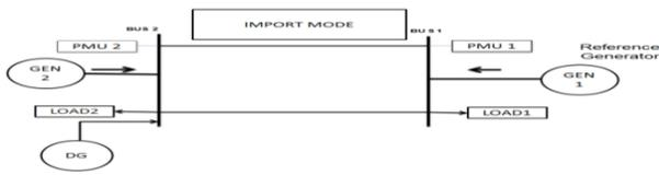
Fig 1: Configuration of the proposed hybrid distributed generation. (Import mode)
