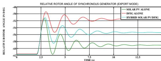
Fig 5: Rotor angle comparison between Solar PV-DFIG and hybrid Solar PV/DFIG (Export mode)
