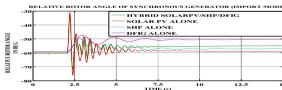
Fig 8: Rotor angle comparison between Solar PV-DFIG-SHP Hybrid Solar PV/DFIG/SHP (Import mode)
