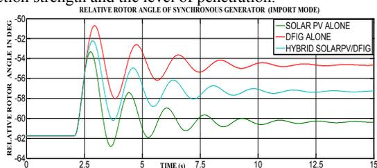
Fig 4: Rotor angle comparison between Solar PV,DFIG and Hybrid SOLAR PV/DFIG (Import mode)
