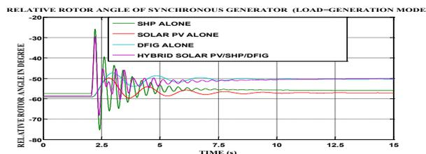
Fig9: Rotor angle comparison between Solar PV-DFIG-SHP and Hybrid Solar PV/DFIG/SHP (Load=Generation mode)
