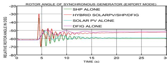
Fig 7: Rotor angle comparison between Solar PV-DFIG-SHP and Hybrid Solar PV/DFIG/SHP (Export mode)
