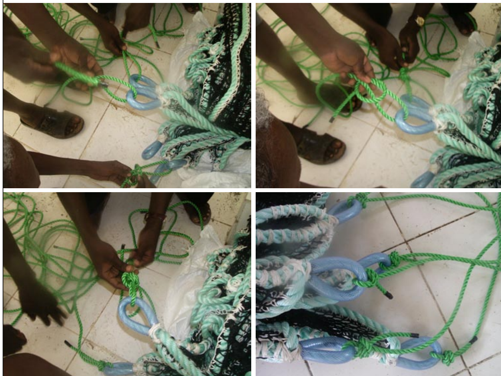
PLATE 43 Knots used for tying the ropes to the loops of the net
