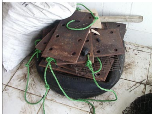
PLATE 44 Ballast weights to be tied to the bottom of the net after it is attached to the cage
