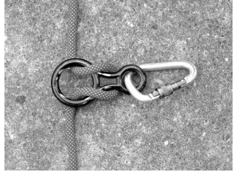
Fig. 2. Attaching the rope to the figure eight. The figure eight is attached to a locking karabiner, which is attached to the harness. The rope going down is where the brake hand should be during abseiling and belaying.
