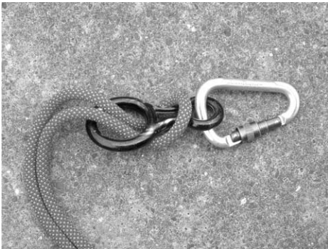
Fig. 3. A different angle. The karabiner is attached below to the harness. In a fall, the figure eight would pull upwards.
