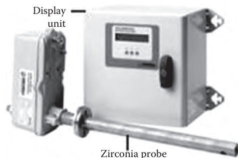
FIGURE 9.13 Oxygen analyser of zirconia type.
