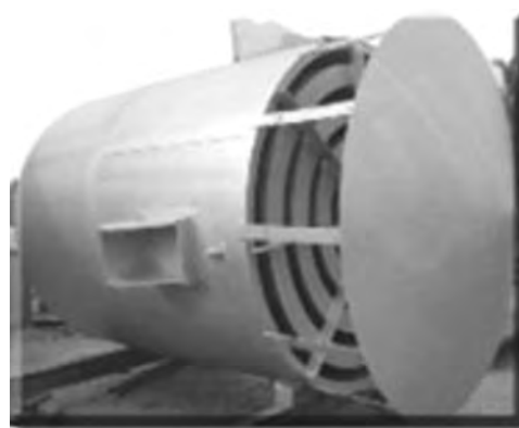
FIGURE 14.6 Safety valve vent silencer in manufacturer's shop.
