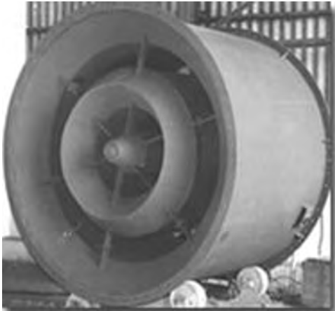
FIGURE 14.7 Fan inlet silencer in manufacturer's shop.
