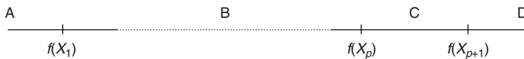
Fig. 7.5 f(z_1) will fall in region A, B, C, or D in the Nelder–Mead algorithm.
