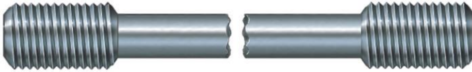
Tension failure of a brittle material
