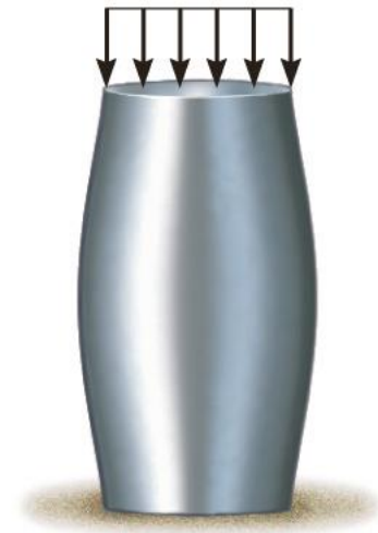
Compression causes material to bulge out
