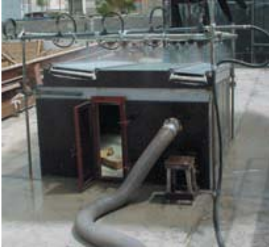
The test chamber, which is capable of being fully sealed, is fitted with an air supply to provide both positive and negative air pressures on the internal face of the roof sample panel.
