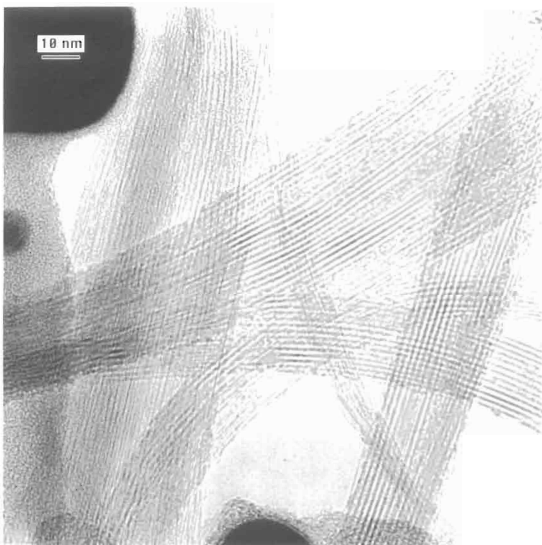
Fig. 2c. Aggregated single-layer nanotubes from soot produced by co-vaporizing Co and Bi.
