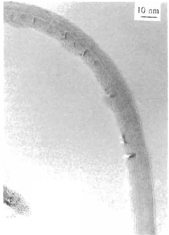
Figure 3. Lattice fringes LF 002 of buckled nanotube particles.
