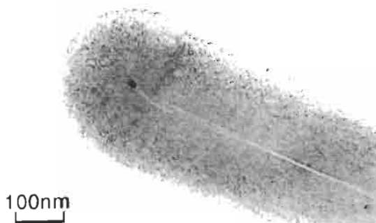
Fig. 2. Vapour-grown carbon fiber showing relatively early stage of growth; at the tip the seeded Fe catalytic particle is encapsulated.
