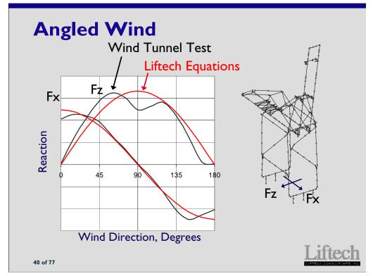
Wind tunnel tests take into account the wind direction.
