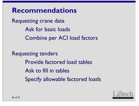
We recommend obtaining the basic loads from the crane manufacturer and combining these loads in accordance with ACI.
