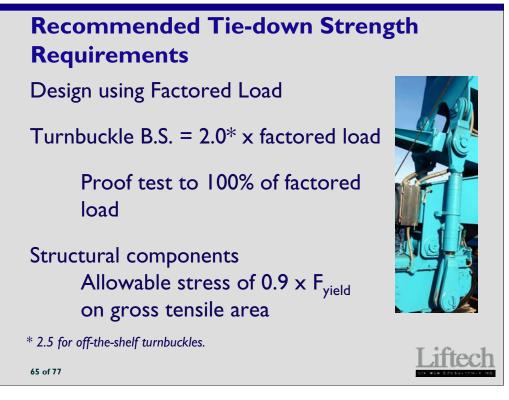
These requirements partially compensate for possible uneven load distribution between tie-downs, if there is more than one per corner. In addition, since the turnbuckle is a mechanical, high-strength, threaded component, it may fail in a brittle manner, unlike the main crane structural components. From our experience, the crane structure is not the "weak link." We recommend that the quay attachment be designed to the same loading and safety factor as the crane tie-down components.
