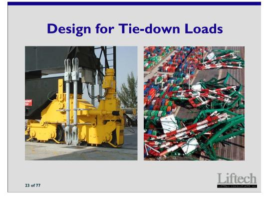
Historically, the most significant design and performance problems occur with the tie-down system. This loading is not well understood by wharf designers and crane manufacturers. Additionally, manufacturers do not understand what parameters are important for the wharf designer.
