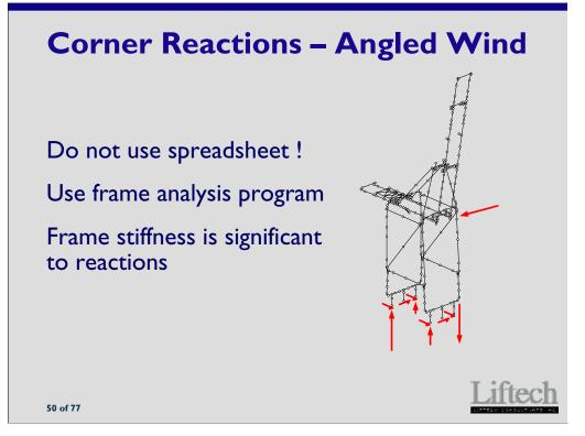
The frame stiffness is significant to the wind reactions.
