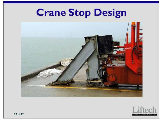
It is important for the designer to understand the basis of the crane stop load that is provided by the crane manufacturer.
