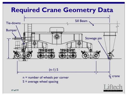
The wharf designer should have an understanding of the crane geometry. At a minimum, the wharf designer should understand these parameters.
