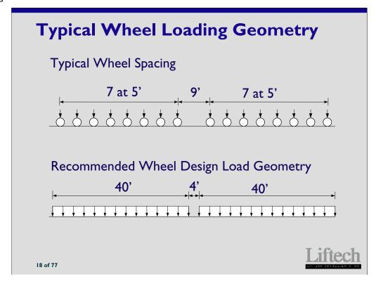
Wheels should be, and typically are, spaced as far apart as possible to distribute the loading into the wharf. The spacing is controlled by the out-to-out bumper distance of the crane (88'6"), and the need for a checker's cab, stowage bracket, or both, at the center of the crane.
