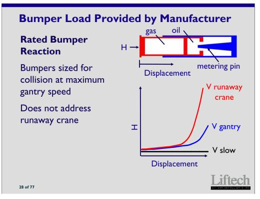
The crane manufacturer typically provides the rated bumper reaction.
