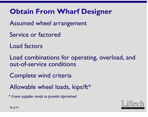
Provide the following to the crane designer so the crane design is consistent with the wharf design.
