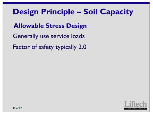
Geotechnical engineers typically design the foundation using an allowable stress approach. Usually a soil capacity twice the maximum service load is designed for. This factor will vary depending on the condition.
