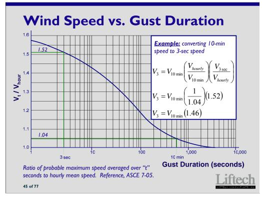
A 3-second gust wind speed is significantly larger than a 10-minute gust wind speed.
