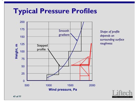
The wind speed and resulting wind pressure profile depends on the surface "roughness" of the area windward of the crane.
