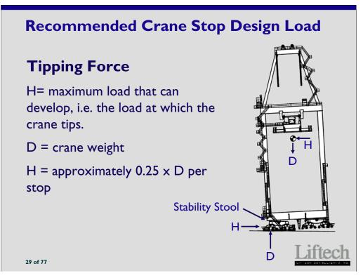
For a runaway crane, the crane stop force will likely exceed the rated bumper force. Localized damage to the crane bumper and support may occur.
