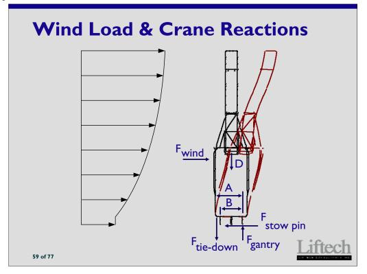
Tie-downs are positioned as close as possible to the end of the sill beam to improve leveraging.
