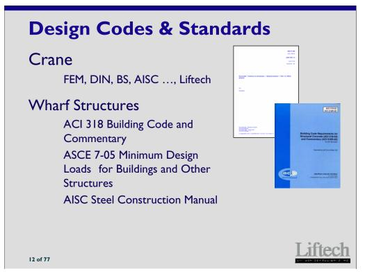
The design codes used for crane structures include a variety of worldwide codes. Typically, several of these codes are used in a crane specification.
