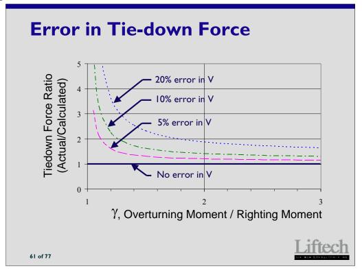
As the ratio of moments increases (bigger uplift), the error in the calculated tiedown force approaches the error in the wind force.
