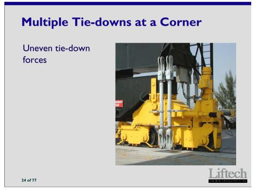
If there are multiple tie-downs at a crane corner, the crane movement, combined with other factors, will cause one tie-down to carry significantly more than its share of the load. If the tie-down system is not ductile, it may fail before the load can be shared by the other tie-downs. This will result in a progressive failure of the tie-downs and crane collapse.
