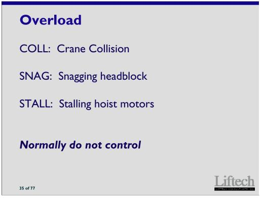
Overloads include the crane colliding with other cranes, the headblock snagging on the ship, and the hoist motors stalling.
