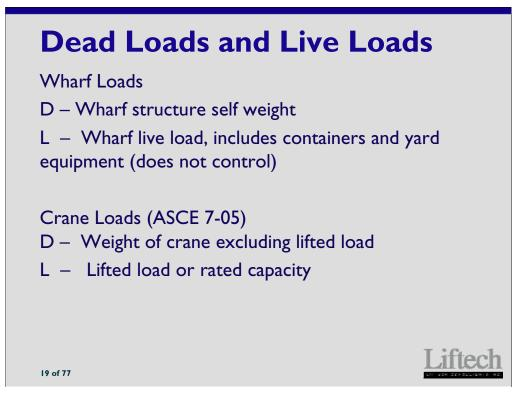
Both the wharf structure and crane weight are considered dead loads because both are accurately estimated. After assembly, it is common to weigh the crane to within a 3% accuracy.
