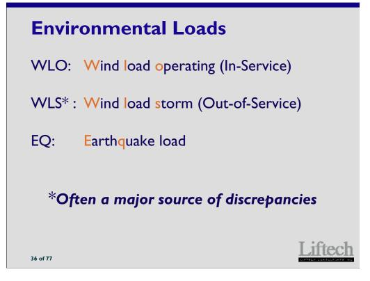
Environmental loads include wind and earthquake loadings.
