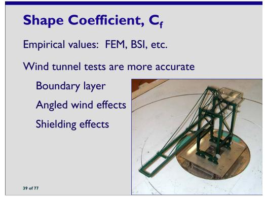
Shape factors for various member shapes have been estimated from many wind tunnel tests. The wind tunnel test shape factors typically differ from the empirical values provided in codes.
