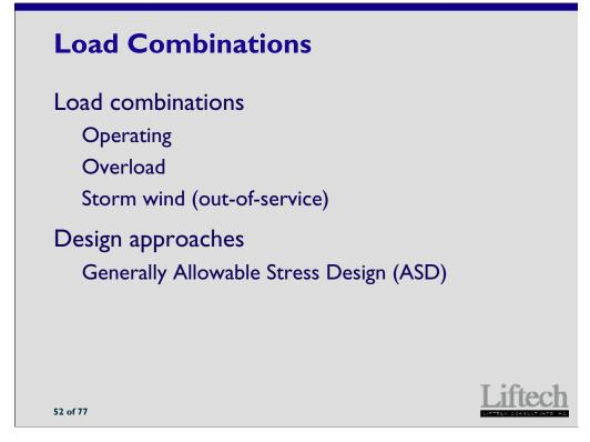
The strength load combinations considered when designing a crane include operating conditions, overload events, and storm wind (out-of-service) conditions.
