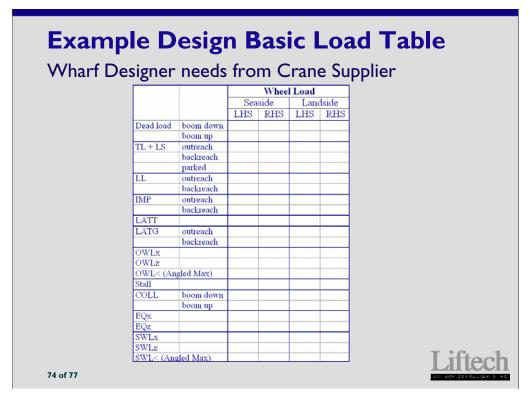
Provide the crane supplier a table containing the desired basic loads for the supplier to fill out and return.
