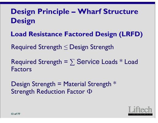
The LRFD design principle is used to design the wharf structure. The required strength is based on the factored service load, while the design strength is based on a reduced nominal strength.
